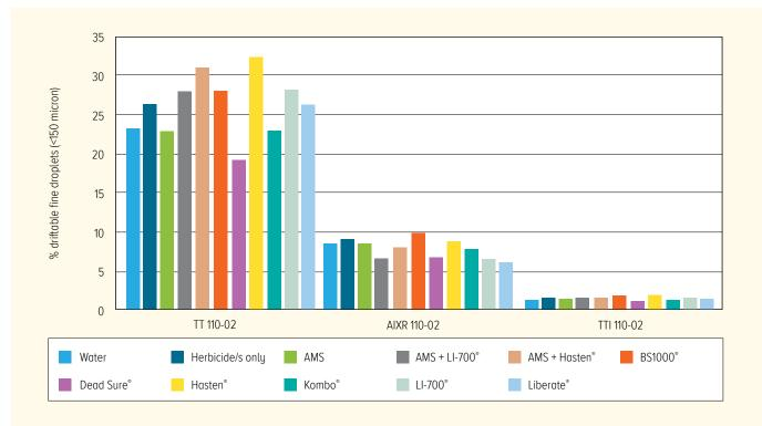
**Figure 1e:** Effect of adjuvant type on the volume of 'driftable fine' droplets (volume mean diameter (VMD) less than 150 micron) produced by three different nozzles.
