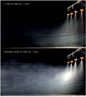
**Figure 1d:** The images above show how two adjuvants with the same nozzle set-up and environmental conditions can result in completely different characteristics of the spray solution. Droplet size is changed causing drift and less product reaching its target. The top image is a spray solution with the surfactant LI-700<sup>®</sup> at 250 ml/100L while the bottom image is Chem-wett 1000 at 200 ml/100L.
