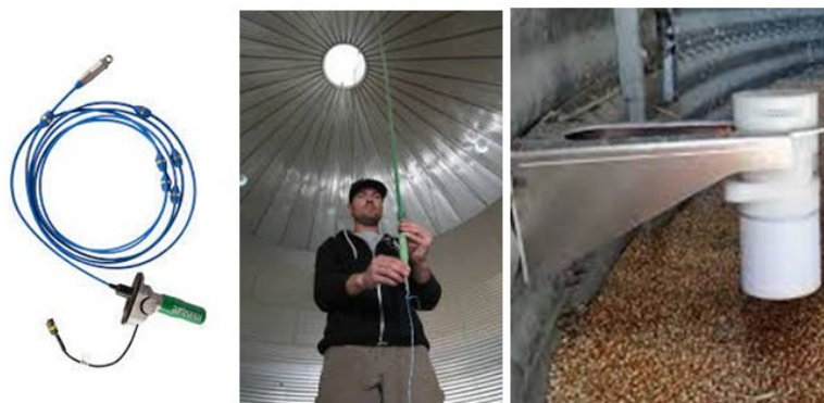
Figure 2. Cable or canister monitoring systems can be located inside a silo to monitor grain temperature, humidity or gases
