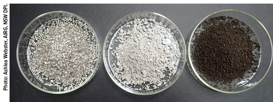
Granular inoculants from left to right: clay granules (attapulgite) coated with peat, clay (bentonite) with rhizobia incorporated and prilled peat.
