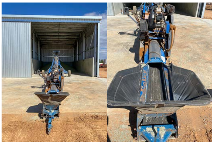
Brandt conveyor belt (left) and hopper (right) used to unload fertiliser into the shed.
