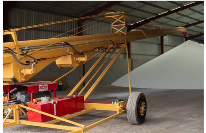
The 36m Sumac 38cm belt auger can unload 6t/minute.
