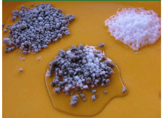
Figure 2: The same piles after 24 hours exposed to high humidity.
