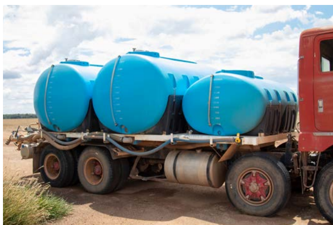
The two nurse trucks each contain two 5000L tanks and a 2000L water tank. Photo: Petrina Ronald
