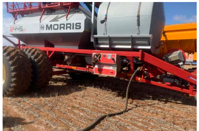
Morris Air Cart with 7000L UAN tank mounted on the front.
