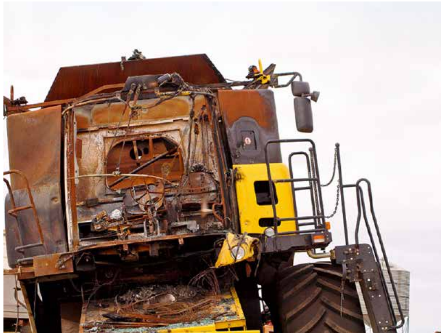
Photo 3: Keeping headers clean can reduce the risk of fire.
