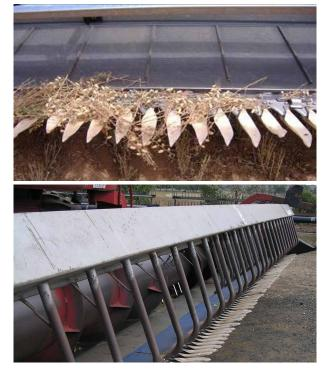
Figure 5: Plastic extension fingers fitted to a Draper front. (Photos: G. Cumming, Pulse Australia)
