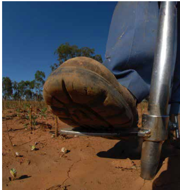
Photo 3: Soil cores need to accurately reflect the main soil type in the paddock being tested.
