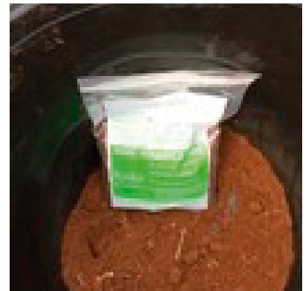
Mix samples in a bucket to get a representative sample of the soil nitrogen profile.
