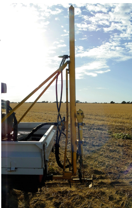
A ute-mounted hydrolic ram probe is ideal for deep N sampling in-season.
