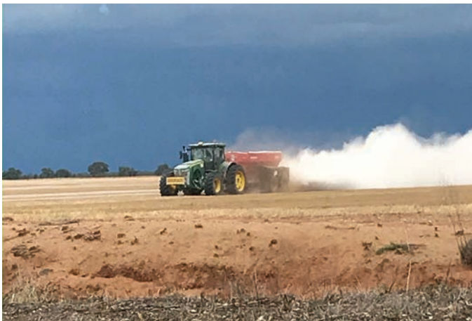
Figure D3: GPS-guided spreading equipment at 'Uah'.
