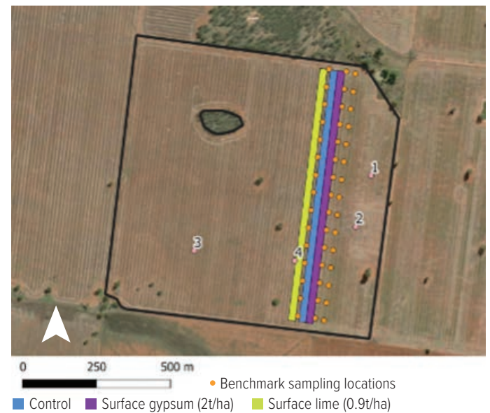
Figure 26: Example strip trials with detailed soil sampling locations to test out different amelioration approaches. Samples are 60m apart. Sampling depth intervals are 0 to 10cm, 10 to 20cm, 40 to 50cm, 60 to 70cm.
