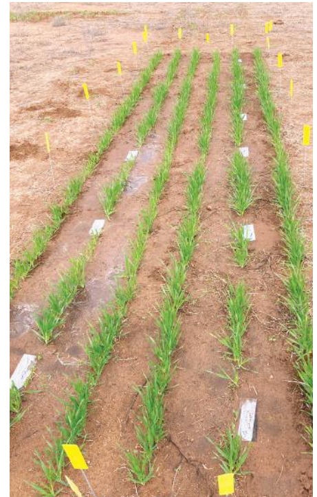
Figure 3: DGT devices used in the paddock to evaluate soil phosphorus status at six weeks after sowing. Barley plants have been removed to facilitate placement of DGT devices.
