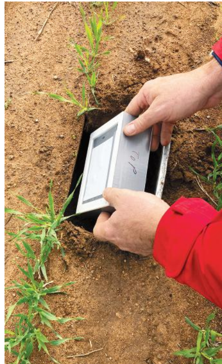
Figure 3: DGT devices used in the paddock to evaluate soil phosphorus status at six weeks after sowing. Barley plants have been removed to facilitate placement of DGT devices.
