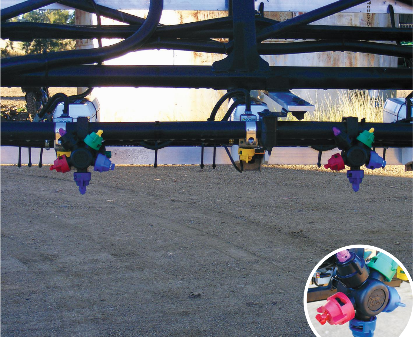
Having a selection of nozzle types available makes it simpler to choose the best one for each situation.
