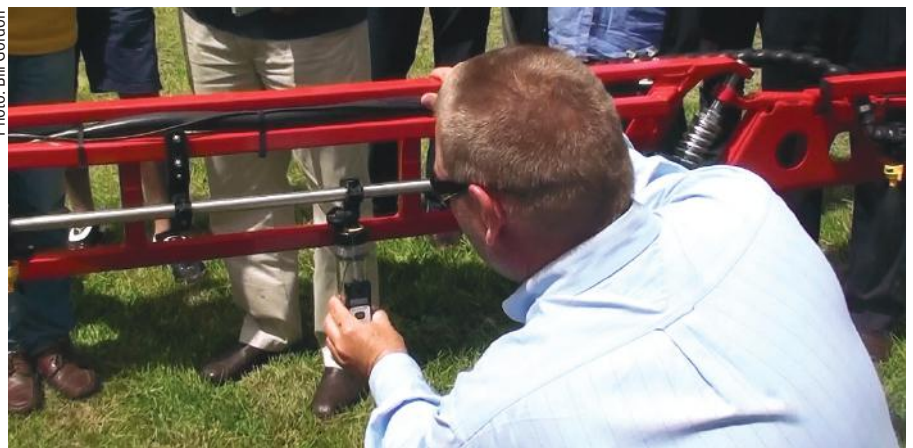
Bill Gordon checking nozzle outputs at an application and drift management workshop in central Queensland.
