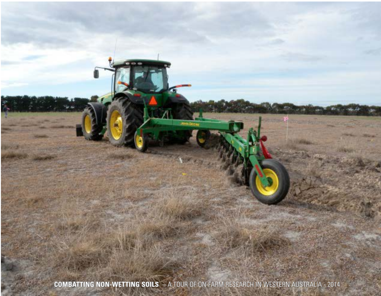
Figure 4: A one pass seeding and ploughing system using a European plough (David Cox)
