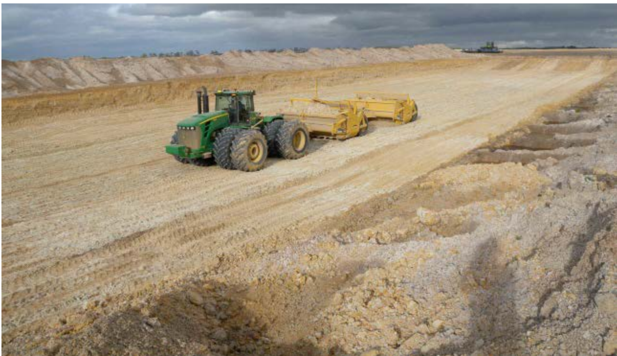
Figure 1 : Claying using a dual carry grader system (Joe DellaVedova) .
