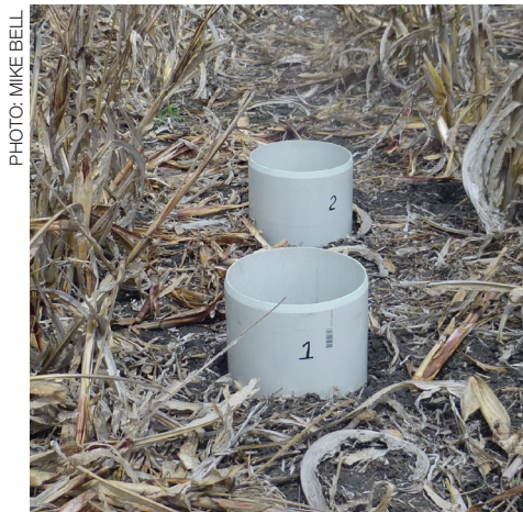
Periodic measurements of nitrous oxide emissions can be measured using manual chambers, as shown in this photo during a fallow after a sorghum crop.
