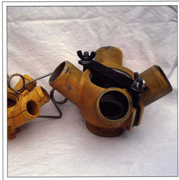
Plate 16 Conversion heads, such as this one for a Connor-Shea airseeder, allow large seeds to be sown with ease.
