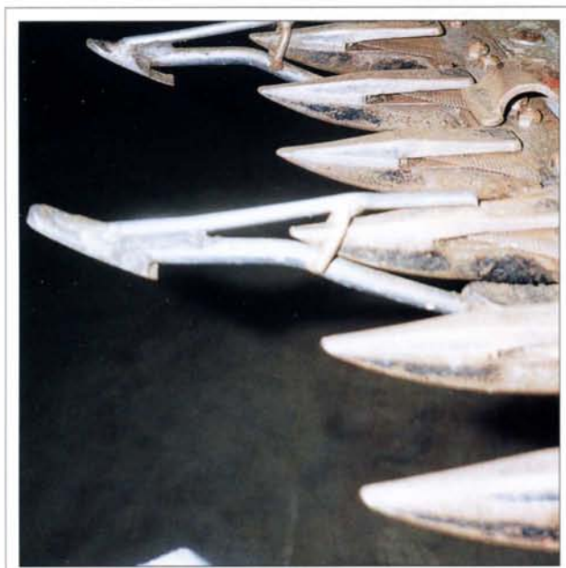
Plate 9.3 Donald Steel Lentil Lifter: with hard shoe welded on front.
