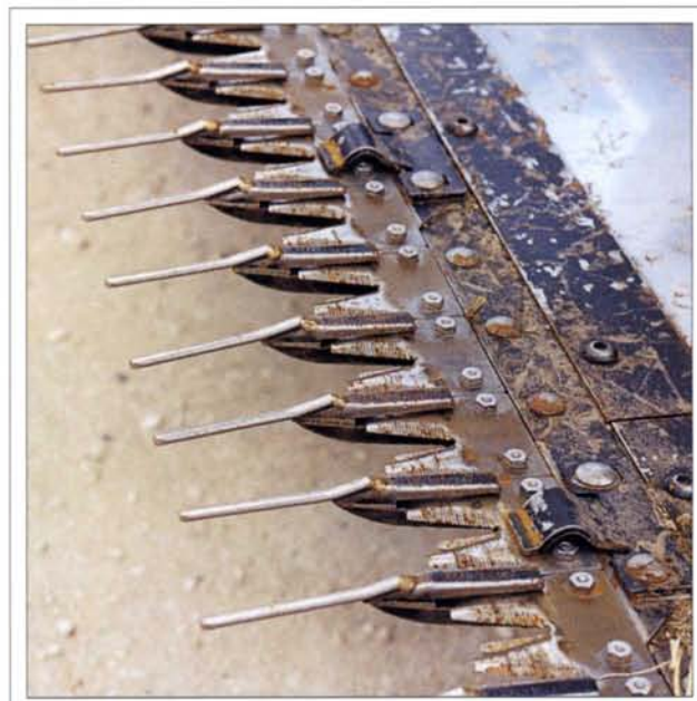
Plate 9.4 Lentil Lifter: 100mm of 6mm round steel welded on to knife guard.
