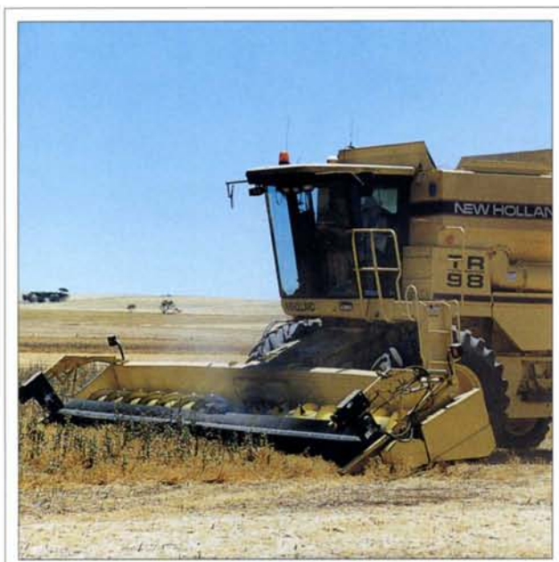
Plate 9.1 Donald Lentil Reel: simple construction; forces material back to table and auger; restricts visibility of knife.
