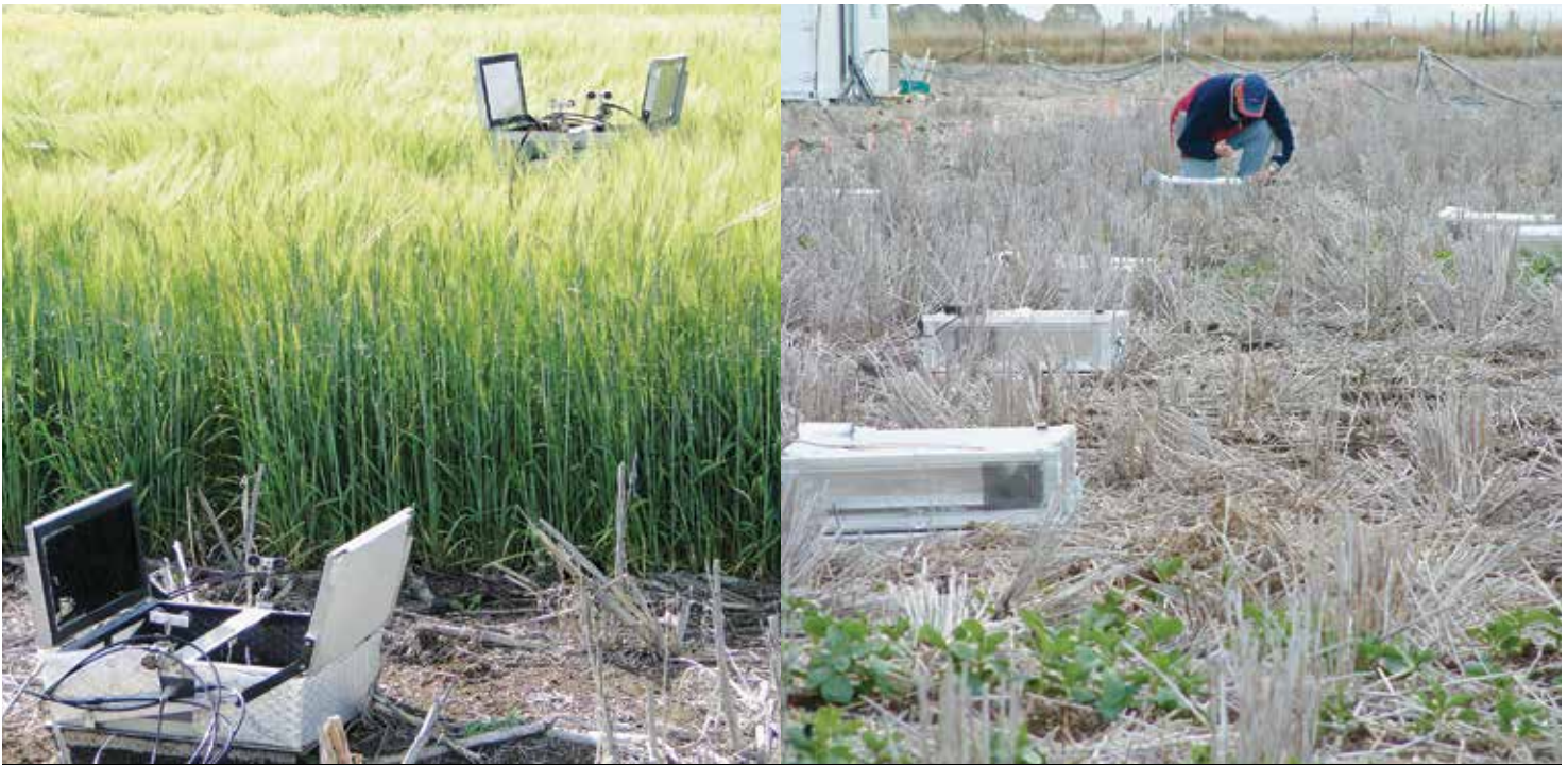
Monitoring greenhouse gas emissions from crops at the NSW Department of Primary Industries at Tamworth. The gases are collected in either automated chambers (above left) or static (manual) chambers (above right).
