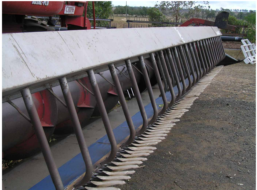
Photo 4: Harvestaire front combined with extension fingers and a blue Vibra-mat.
