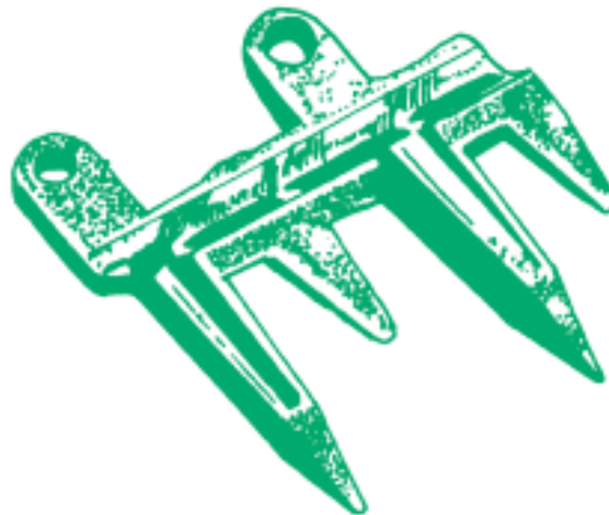
Figure 1: Four-finger guards to reduce vibration.
