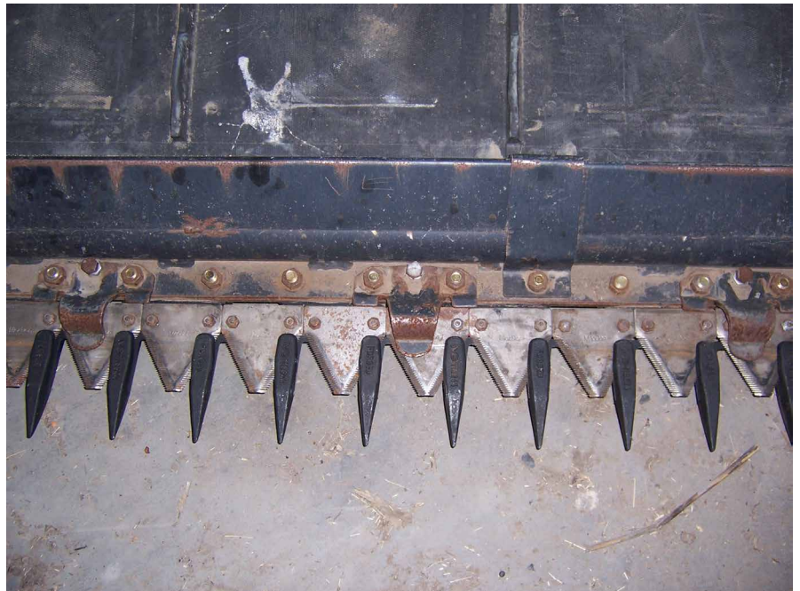
Photo 2: Short fingers on a flex-front.
