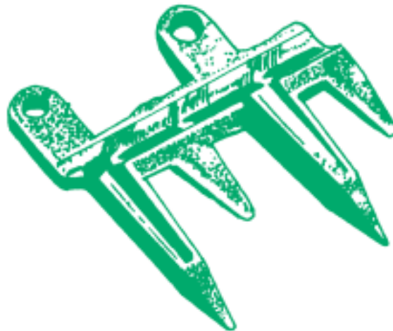
Figure 1: Four-finger guards to reduce vibration.
