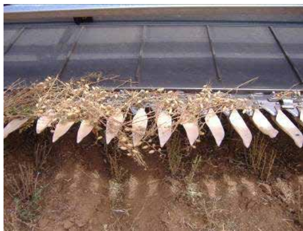
Photo 3: Plastic extension fingers fitted to a draper front.
