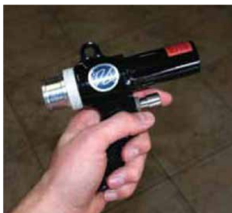
Figure 6: A blow/vac or air venture gun is the best applicator for inert dusts. (Photo: C. Warrick, Kondinin Group)
