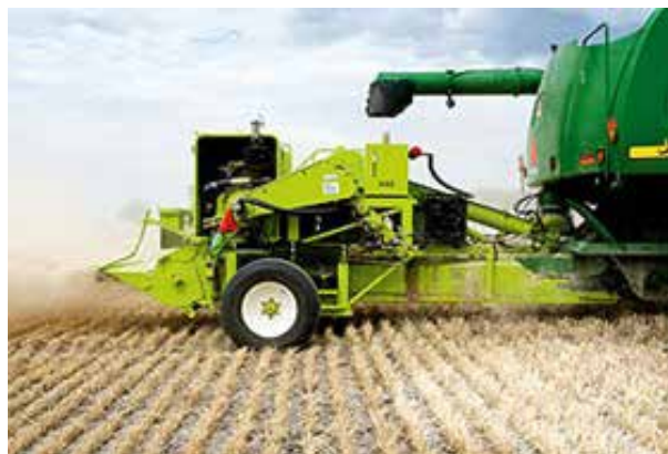
Photo 4: Harrington seed destructor at work.
