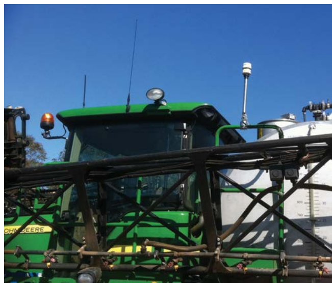
The location for the 'on the go' weather station that Robin has found to ensure the data is collected reliably. Photo: Robin Schaefer
