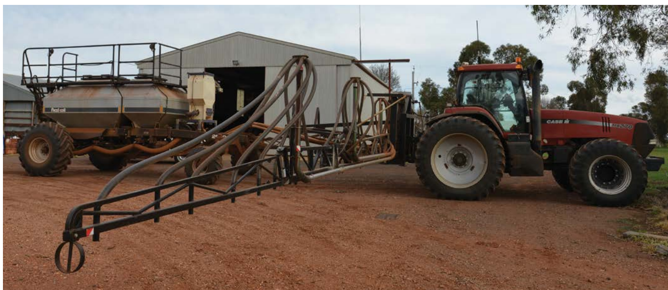
Using the air-cart and fertiliser boom allows up to three products to be applied at variable rates. The boom heads are the same as the airseeder and distribution is spaced between the crop rows. Photo: Emma Leonard
