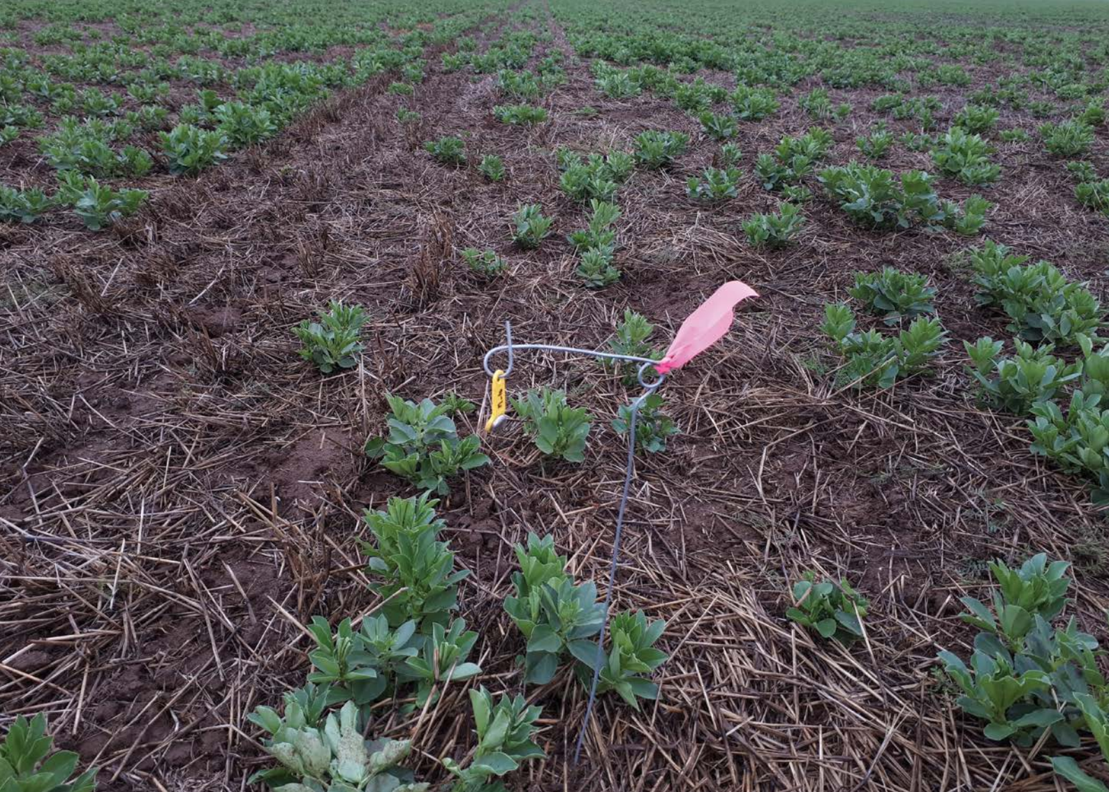
A coin sized temperature sensor suspended 50cm above the ground in a faba bean crop at the mid-north site near Mintaro, SA. Photo: CSIRO
