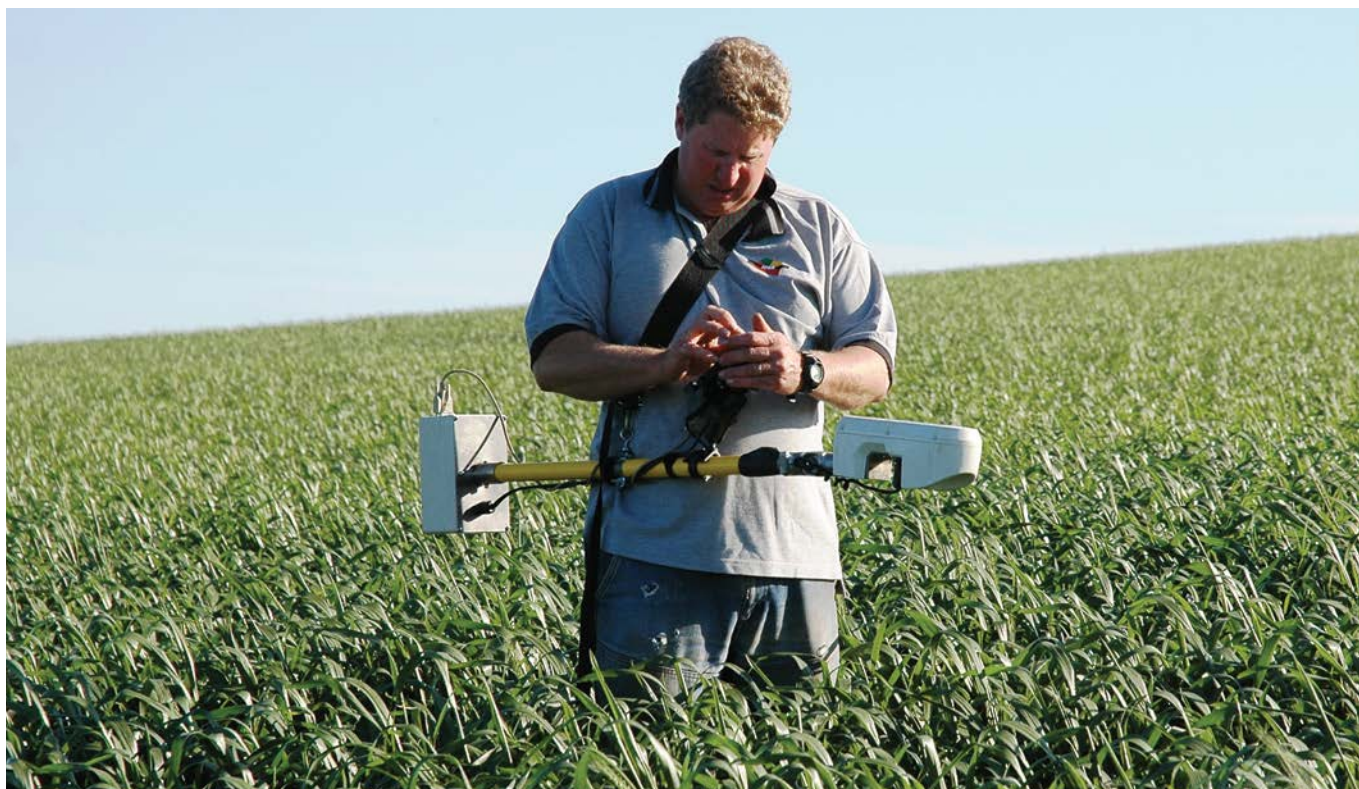
Mark uses a handheld biomass sensor to compare crop reflectance of the N-Rich strip against the adjacent crop to establish the range of N requirement. Photo: Emma Leonard
