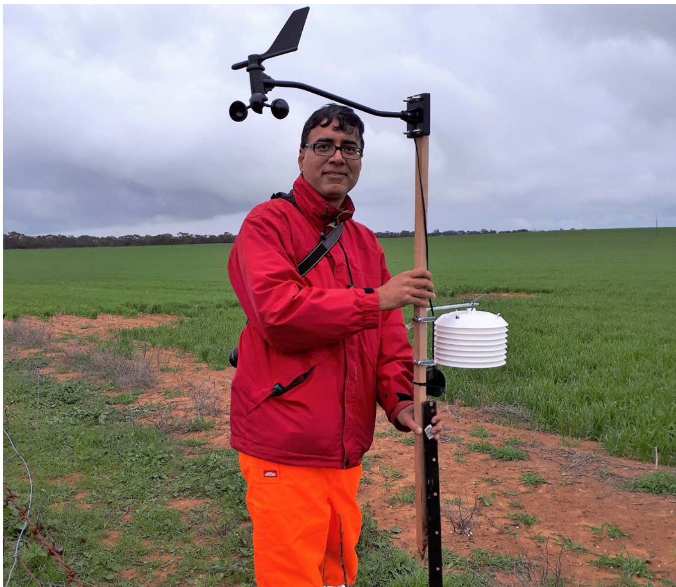
Uday Nidumolu installing a mini weather station at the Jabuk trial site, SA Mallee. Photo: CSIRO
