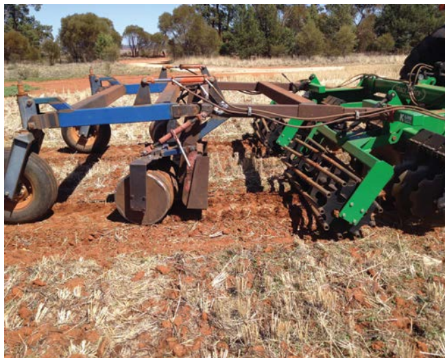
The addition of a roller set at about 45 degrees to the track and a hydraulically adjustable scraper to a commercial track renovator which is used judiciously to reinstate smooth, hard tracks. Photo: M Pfitzner
