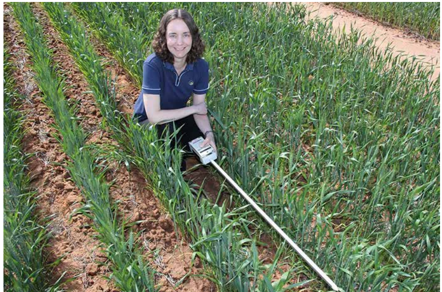
Photo 1: Measuring light availability to the inter-row space in wheat with a Sunfleck Ceptometer
