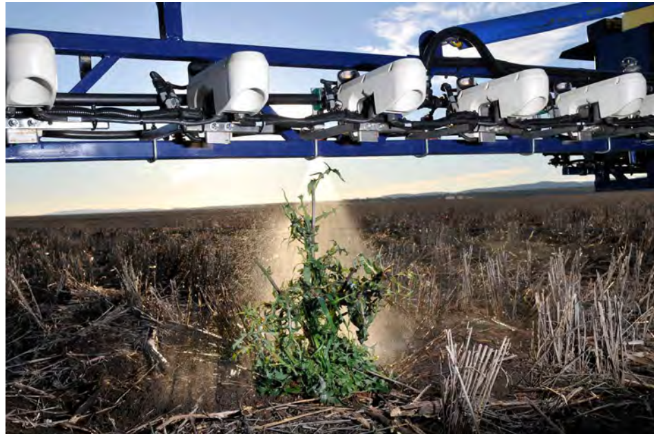
Figure 15: Selective sprayer technologies use optical sensors to turn on spray nozzles only when green weeds are detected. (Photo: CropOptics)
