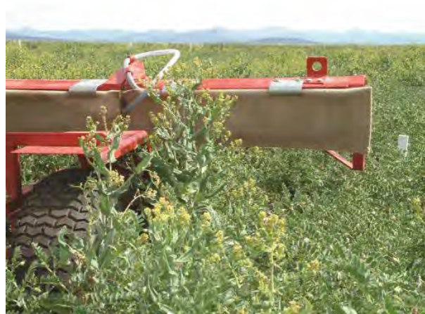
Figure 5: Blanket wipers use a sheet (blanket) moistened with herbicide to wipe the weeds above the crop. (Photo: A. Storrie)
