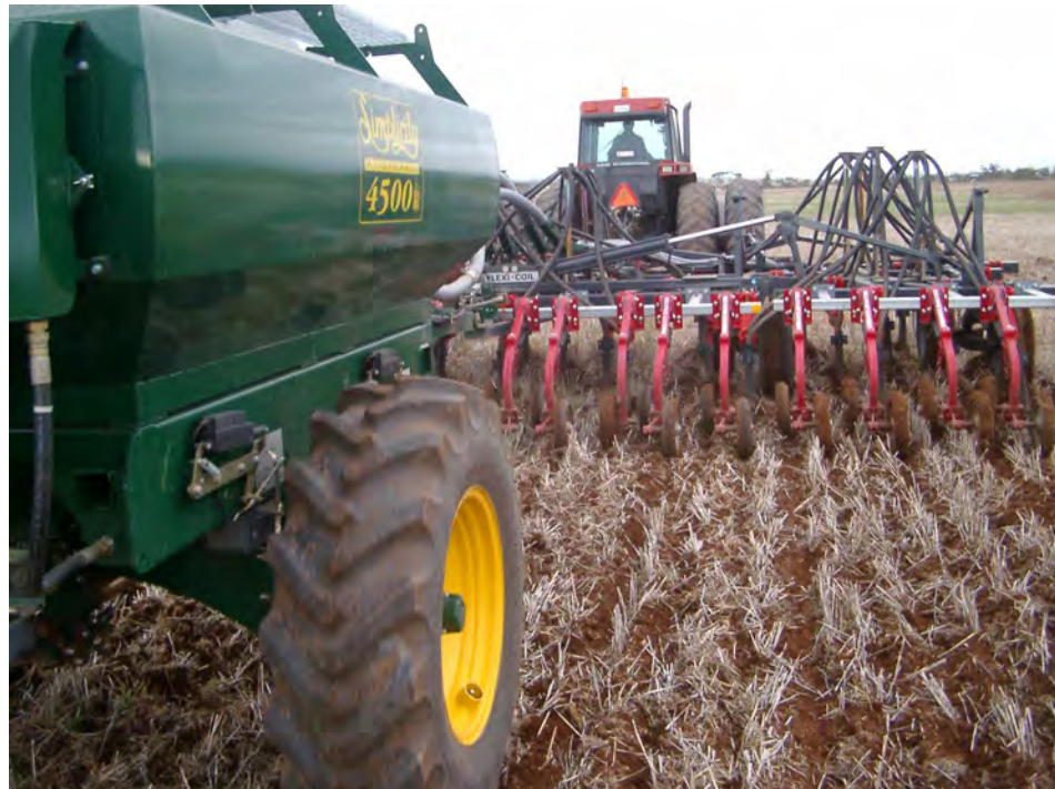
Figure 16: Seeder calibration is important for precise seed placement and seeders need to be checked regularly during sowing. (Photo: Rohan Rainbow)
