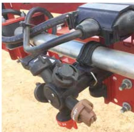
1. Improved electronics and fully protected wiring on a new Case Patriot sprayer (2018). Note the modular nozzle body turret 'clip and play' components giving flexibility for endless configurations.
