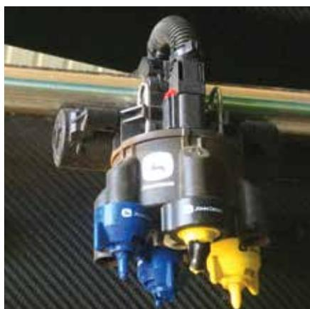
2. John Deere's ExactApply™ is a good example of the latest engineering and modularity with multiple spraying systems within one carousel unit. It contains a standard spraying system, multi-step system and PWM.
