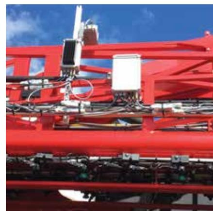
3. The Agrifac multiple spraying systems with standard, twin fluid, PWM – 100hz, and new camera (back view) for weed-recognition technology.
