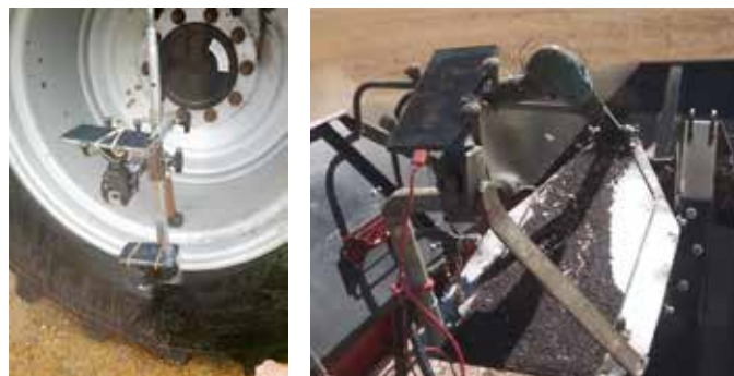
FIGURE 1: The WheelCam attached to a Case header (left) and the GrainCam attached to the bubble auger (right).
