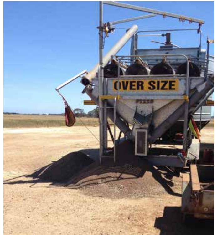
A rotary screen cleaner can be used to scalp small conical snails from canola.
