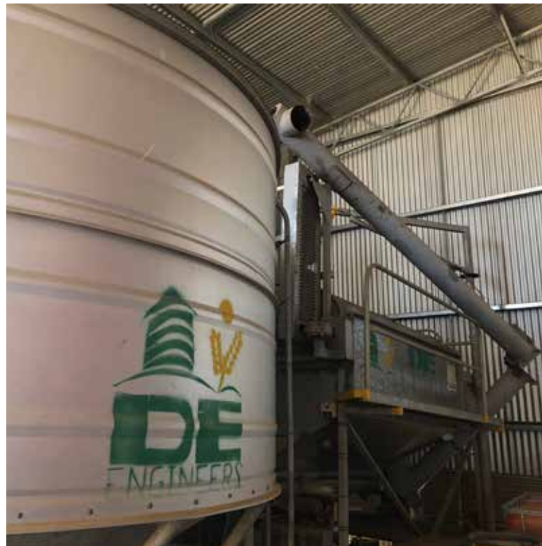
A DE Engineers grain cleaner is used to remove snails from canola at harvest.
