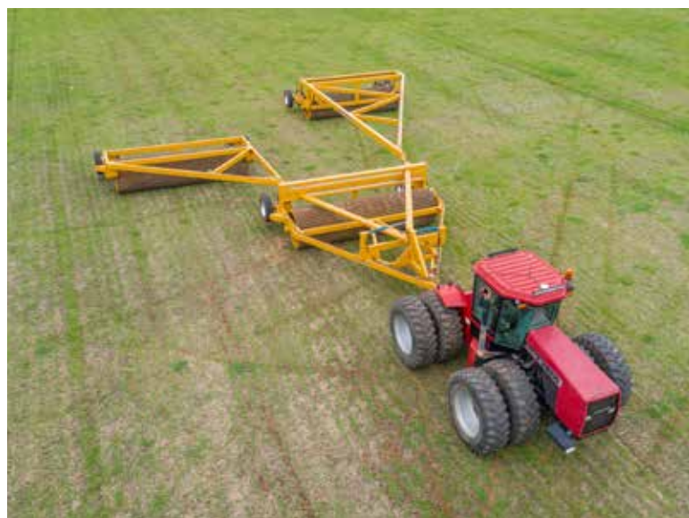
A stone roller used for crushing stubbles. Stubble management is normally done before seeding.
