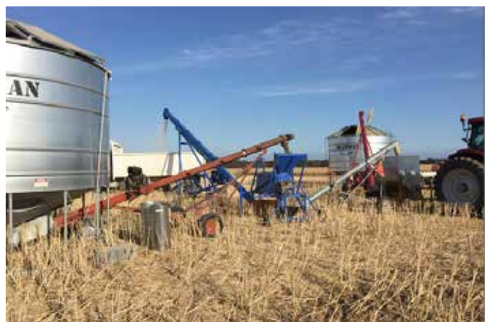
Grain cleaning set-up during harvest: grain goes from storage silo into grain cleaner, then through the snail roller and finally into a clean silo or straight onto a truck.
