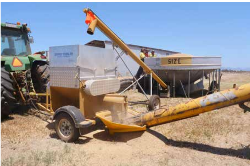
The single model snail roller used to remove snails from barley in the 2018-19 SCF demonstration. PHOTO: SCF
