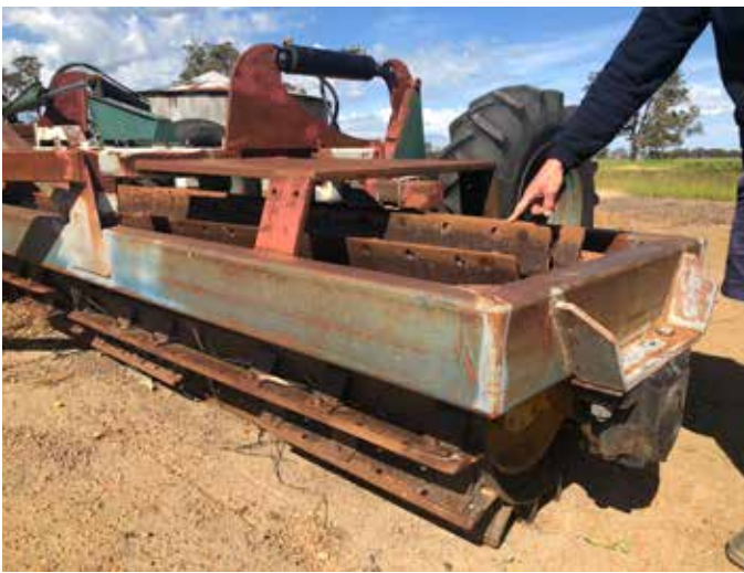
A home-manufactured stubble cruncher showing blades that break up stubble and incorporate it into the ground, disturbing the snails' habitat.
