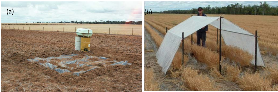
Figure 2. (a) Wetting up for DUL determination and (b) rainout shelter used for CLL determination.
