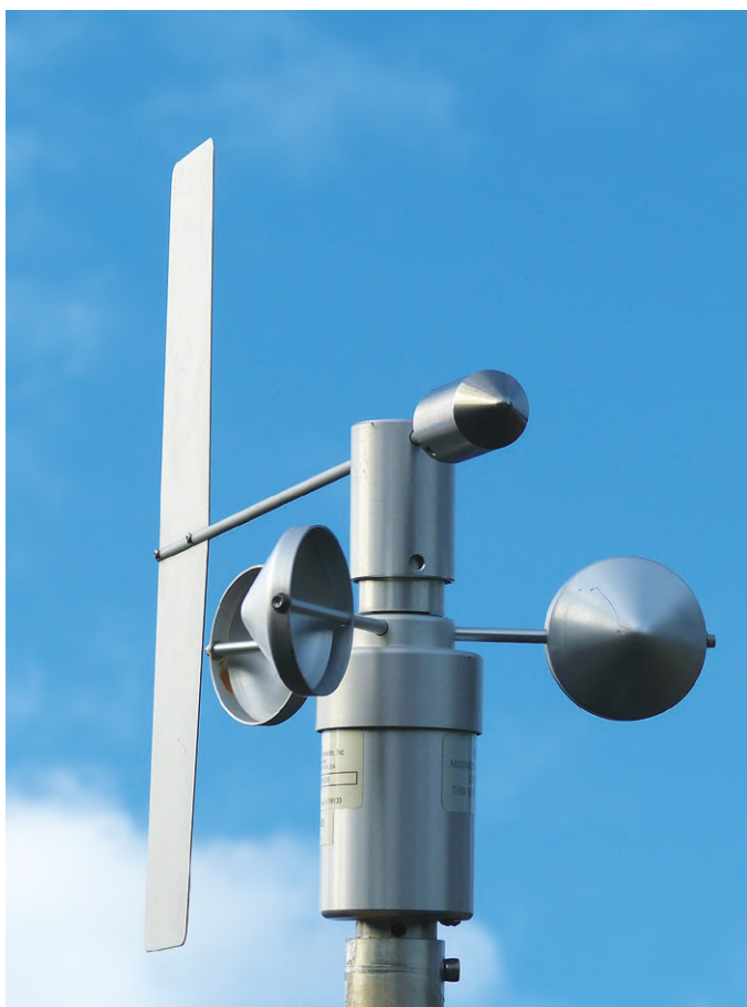
Figure 26: A high quality cup and vane anemometer.
