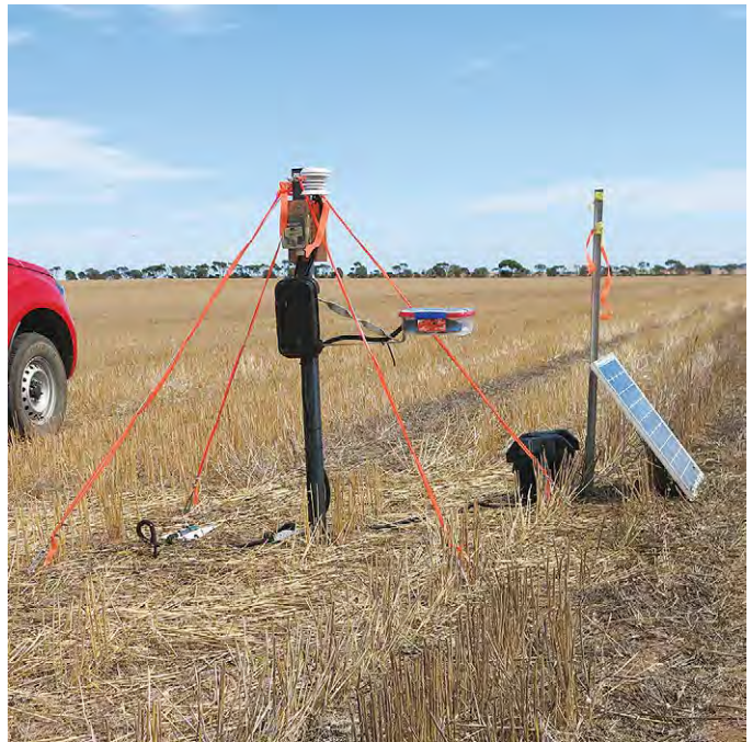
Figure 3.9: Time-lapse camera and weather station for monitoring snails.
