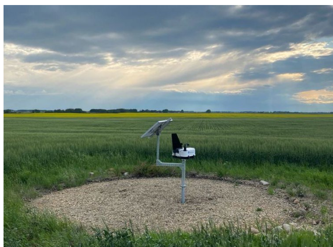
Figure 1. A SporeScout unit in wheat. The unit is powered by a solar panel on the left side, and a black wind vane keeps the intake nozzle consistently pointed into the wind for optimal air sampling.
