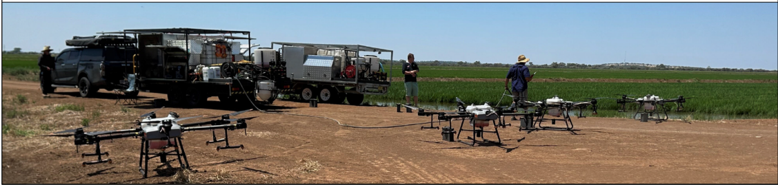
Figure 2. Green on green detection of a weed in rice and integrated into spray drones. Drift was measured to be less than 5m during application.
