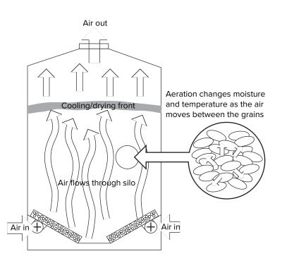
**Figure 2:** Cooling–drying fronts in the aeration process. (C. Newman, Department of Agriculture and Food, WA).
