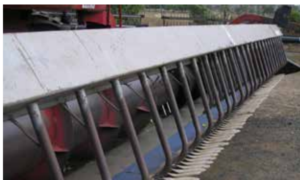
Figure 2: Harvestaire front combined with extension fingers and a blue vibra-mat. (Photo: G. Cumming, Pulse Australia)
