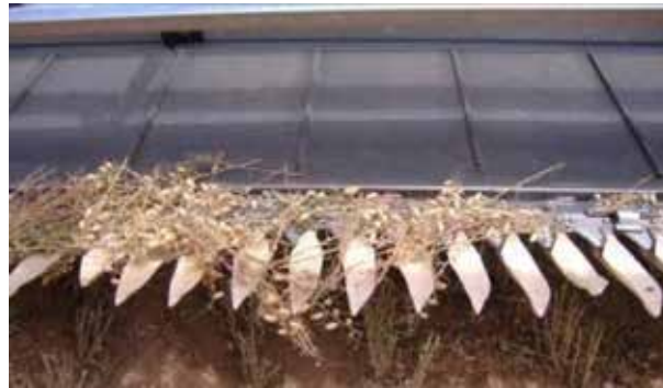
Figure 3: Plastic extension fingers fitted to a Draper front. (Photo: G. Cumming, Pulse Australia)
