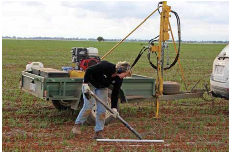
Photo 3: To be meaningful, soil sampling needs to take into account spatial variation in soil condition. Differences in soil type, nutrient status and other soil properties may be exhibited within a paddock.
