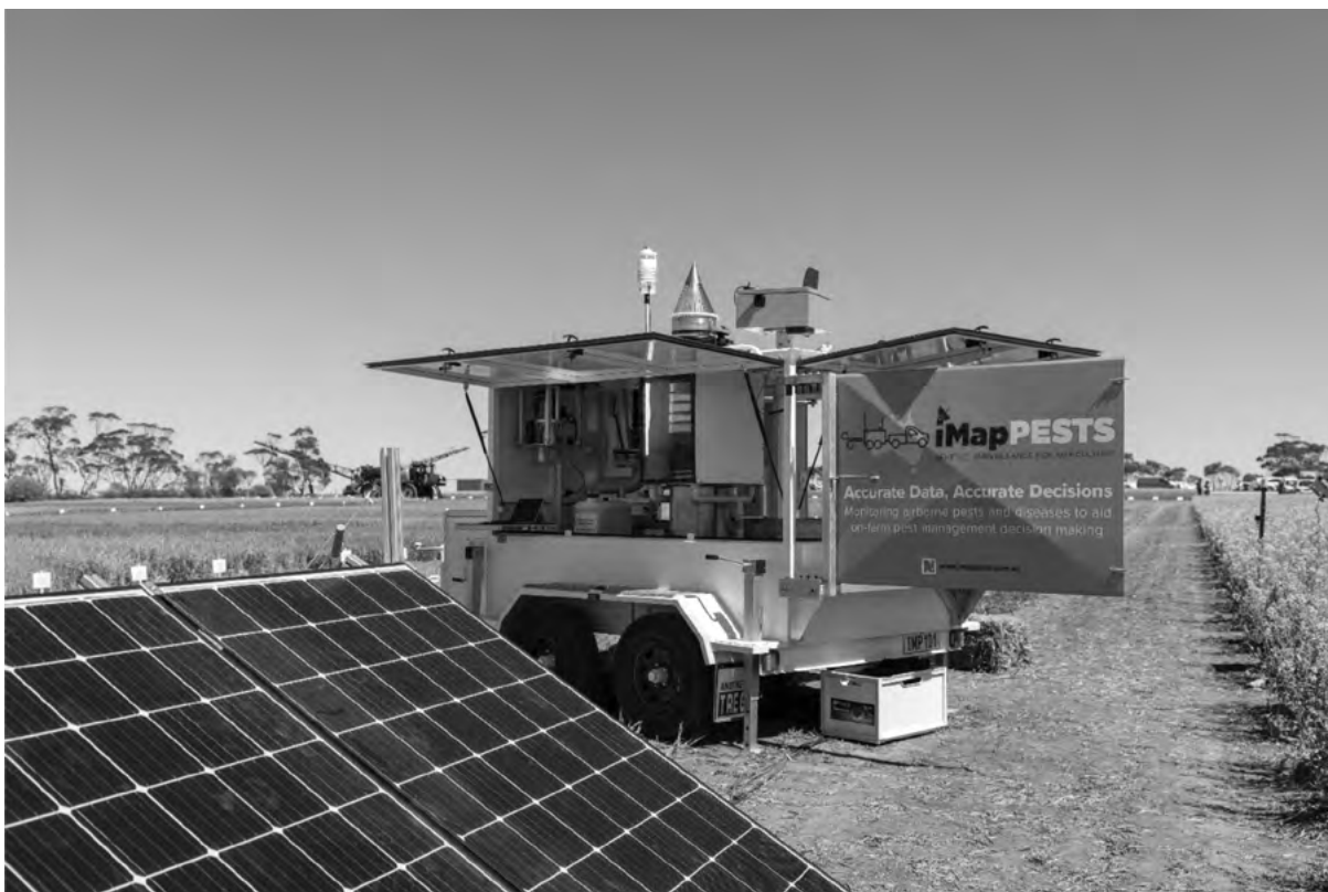
Figure 2. The iMapPESTS sentinel prototype (which is the first of six such units to be developed as part of iMapPESTS) situated at the Hart Field Site in South Australia’s Mid North region during spring in 2019. Internal components visible when the unit is open, and solar panel array to charge its battery banks in the foreground.
