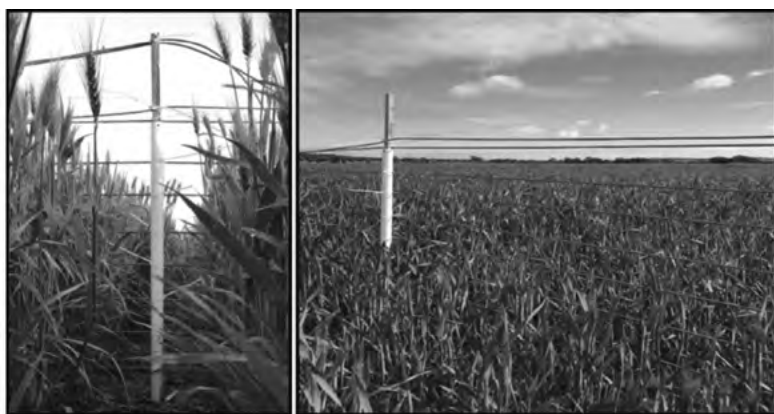
Figure 3. Distributed Temperature Sensing (DTS) fence. (left) Fence support pole. (right) DTS fence at the trial site (cables).
