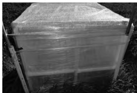
Figure 1. Frost exclusion chamber (photo by Mick Faulkner).
