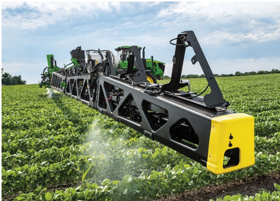
Figure 1. See and Spray Ultimate from John Deere, a green-on-green spot spraying solution. Source: Agfri (2022).
