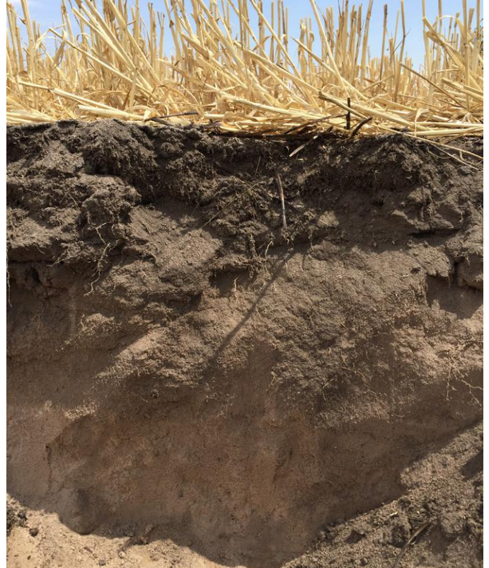
b) About 20cm of sand (water repellent) over dense next layer that is too hard to dig. pH testing required.
