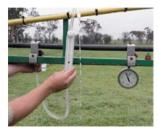
Set the machine to manual pressure, or use the test speed or auto calibration function to set an application volume (L/ha) and speed (km/h) that will give you a known pressure at the nozzle. For example, if you are
