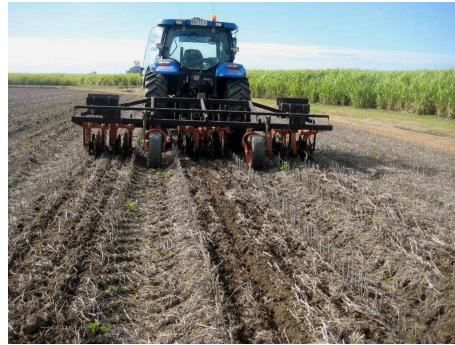
Figure 1: Zonal or strip tillage applied to the inter-row of soybean crop stubble using a 'Soil Soldier'. The objective is to encourage better rainfall penetration and create a zone that is conducive to rapid germination of cane sets planted in a dual row between the three soybean rows on the bed, whilst causing minimal disturbance to the structure of the beds and maintaining controlled traffic zones. (Photos: Alan Munro, Woodford Dale, NSW)
