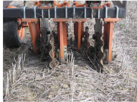
Figure 1: Zonal or strip tillage applied to the inter-row of soybean crop stubble using a 'Soil Soldier'. The objective is to encourage better rainfall penetration and create a zone that is conducive to rapid germination of cane sets planted in a dual row between the three soybean rows on the bed, whilst causing minimal disturbance to the structure of the beds and maintaining controlled traffic zones. (Photos: Alan Munro, Woodford Dale, NSW)
