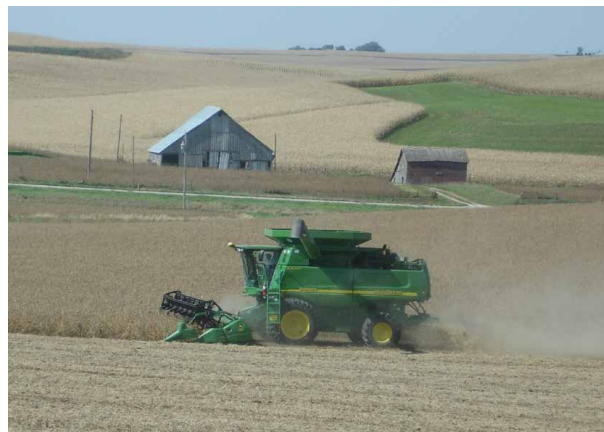
Figure 1: John Deere's STS 9760 with rotary threshing and separation shown in Iowa soybeans. The two types of combine harvesters in Australia—rotary and walker-or drum-type - are now all fully imported. Rotary separators dominate the modern market. John Deere no longer offers walker-types. In Australia we call such machines “headers” but the fact that these machines are all imported and take in more than just the crop heads may spell the eventual end of that name. (Photo: Australian Oilseeds Federation)
