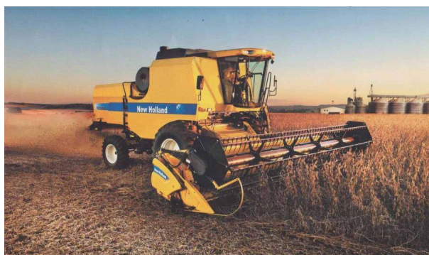
Figure 2: New Holland TC 5090 combine made in Belgium with five walkers shown. Walker separation is preferred in much of Europe where crop conditions are moister and farmers want the longer crop straw for baling. Lately there has been a move to hybrid machines in Europe for higher capacity at some sacrifice in straw quality. (Photo: Australian Oilseeds Federation)
