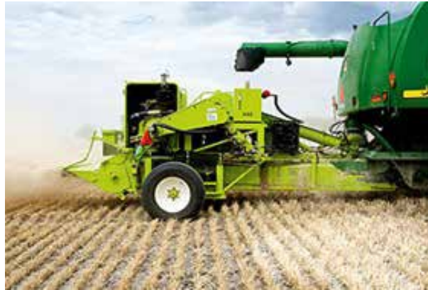
Photo 7: Harrington Seed Destructor at work.
