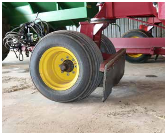
The Vermeersch family advises putting stubble guards on the front of the tyres, as they have replaced every single tyre on the front of the bar in the 2018 season.
