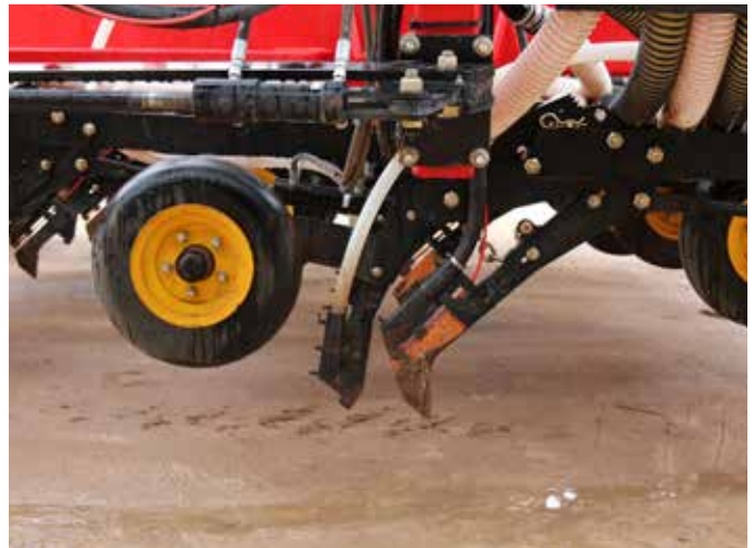
To manage the trash flow around the two tynes, the Cowans harvest a few degrees off their seeding lines so trash does not bunch up on the front tyne.
