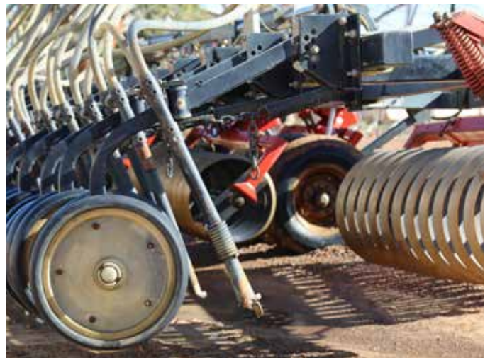
On their freshly mouldboarded paddocks, the Warrs use a Manutech set-up with Flexi-Coil coil packers followed by a seeding boot and a wide press wheel behind that. . PHOTO: CUSSONSMEDIA
