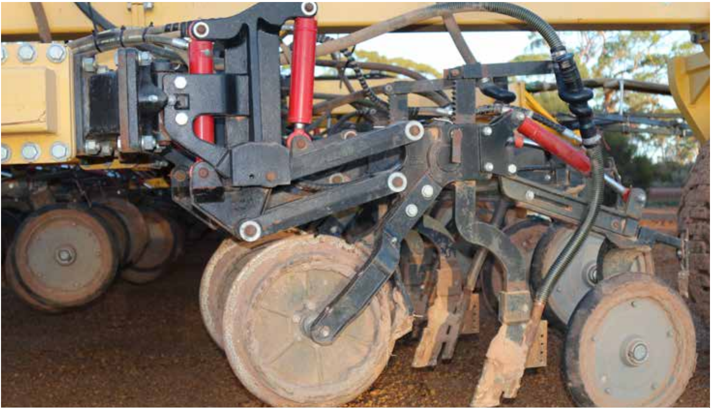
On the Shadbolts' Moisture Manager™ bar, the parallelogram, breakout tyne pressure and press wheels are all independently hydraulically controlled.
