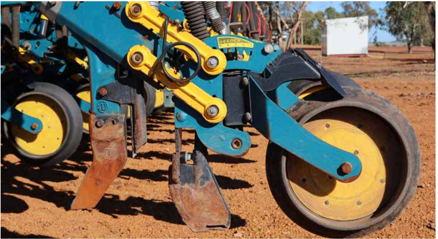
Lawson Grains uses the same tynes, points and seeding boots for all crops, so the seeding bars require minimal changes between the different crop types.
