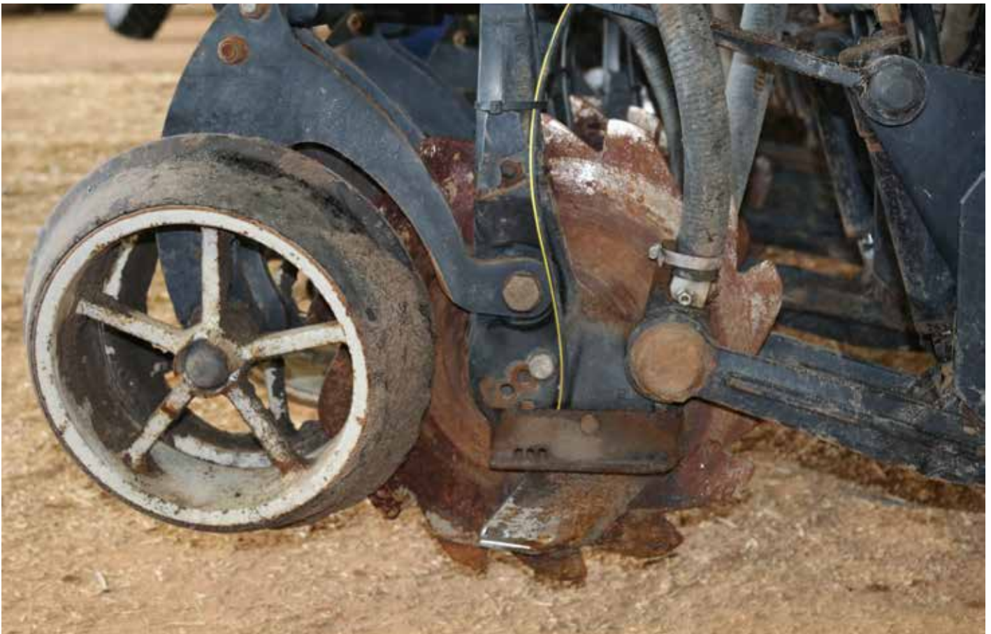
Paul has found the seed and fertiliser separation to be excellent because there is a physical disc separating the two blades that deliver the seed on the left side and fertiliser on the right.
