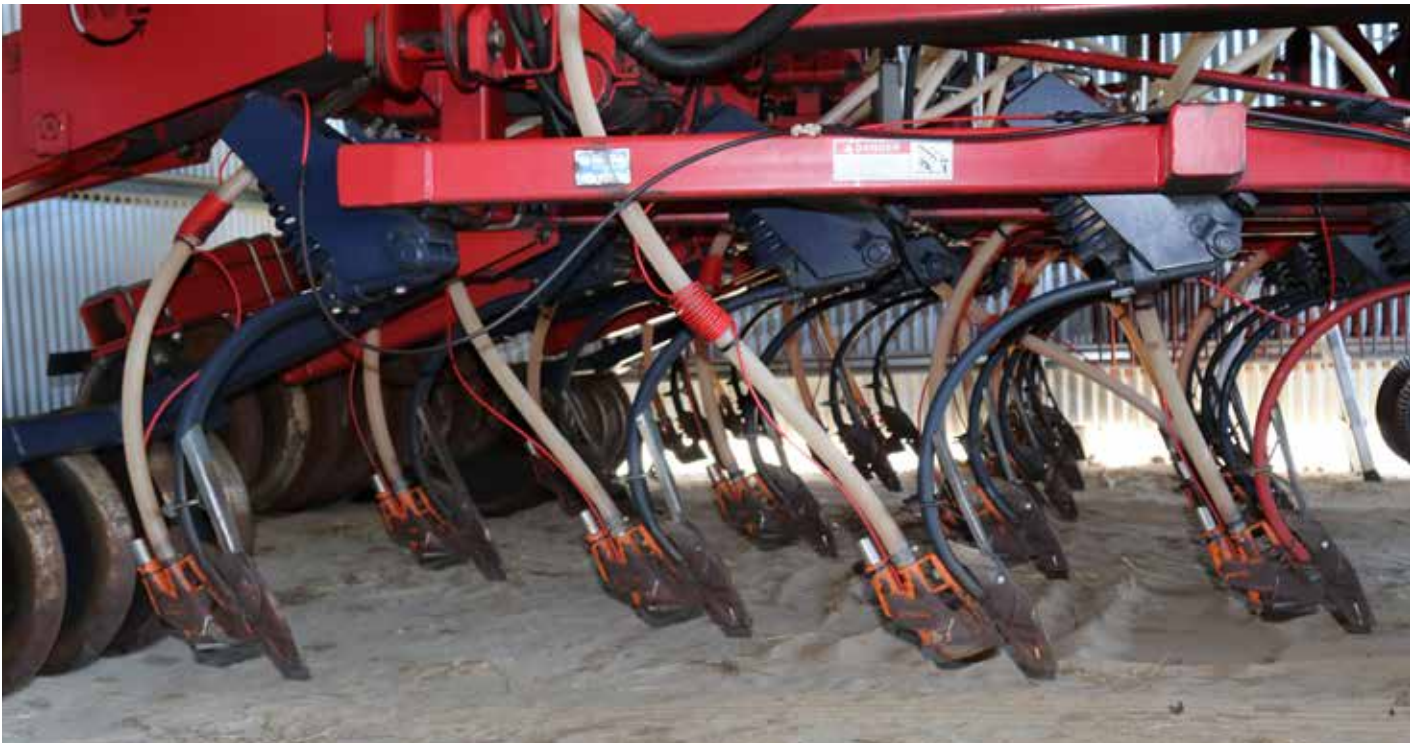
While they initially opted for Root Boot splitter boots to eliminate issues with sealing over in the bottom of the furrow and slotting, Lee says they have also found their 25cm spacing and splitter boot combination to be excellent for early weed competition.
