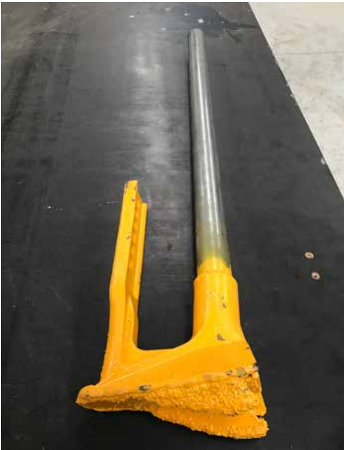
Kirk believes using a purpose-built DBS Stiletto boot is a much better system than a banana boot or s-canola boot. In their system, the original DBS closing tool is removed and the Stiletto boot becomes part of the closing tool.
