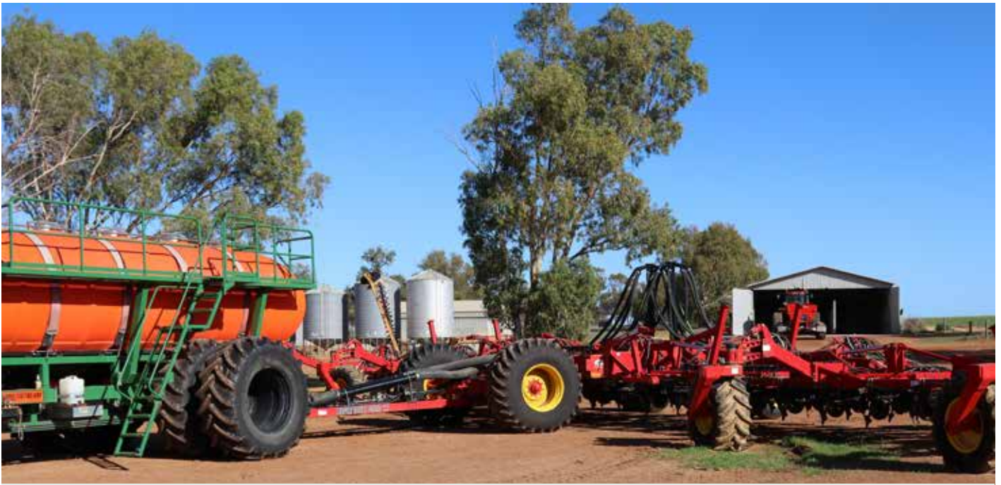
The Warrs' rig includes a 22,000L Ausplow box split into five compartments. In 2019 Brett is looking to add section control to reduce operator error. PHOTO: CUSSONSMEDIA
