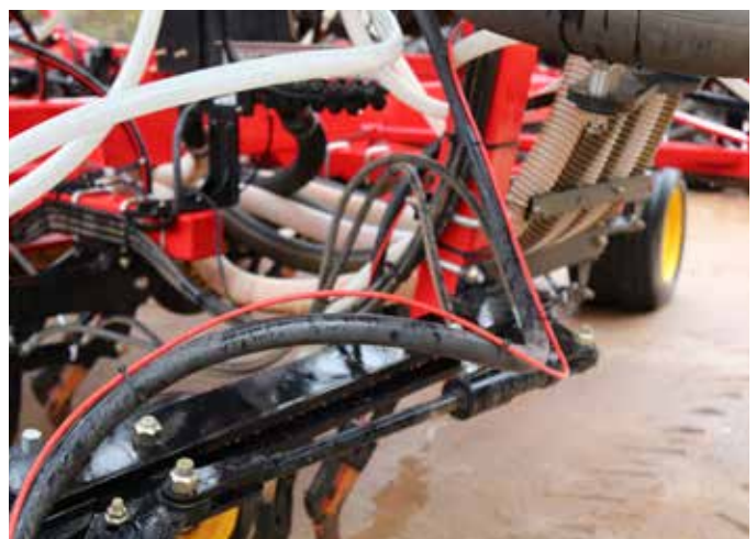
After having three liquid setups on bars, the Cowans have found the best method is to run the main hoses up to the heads and then break them off from there, so they have the smaller lines with the friction hose running to the seed hose.
