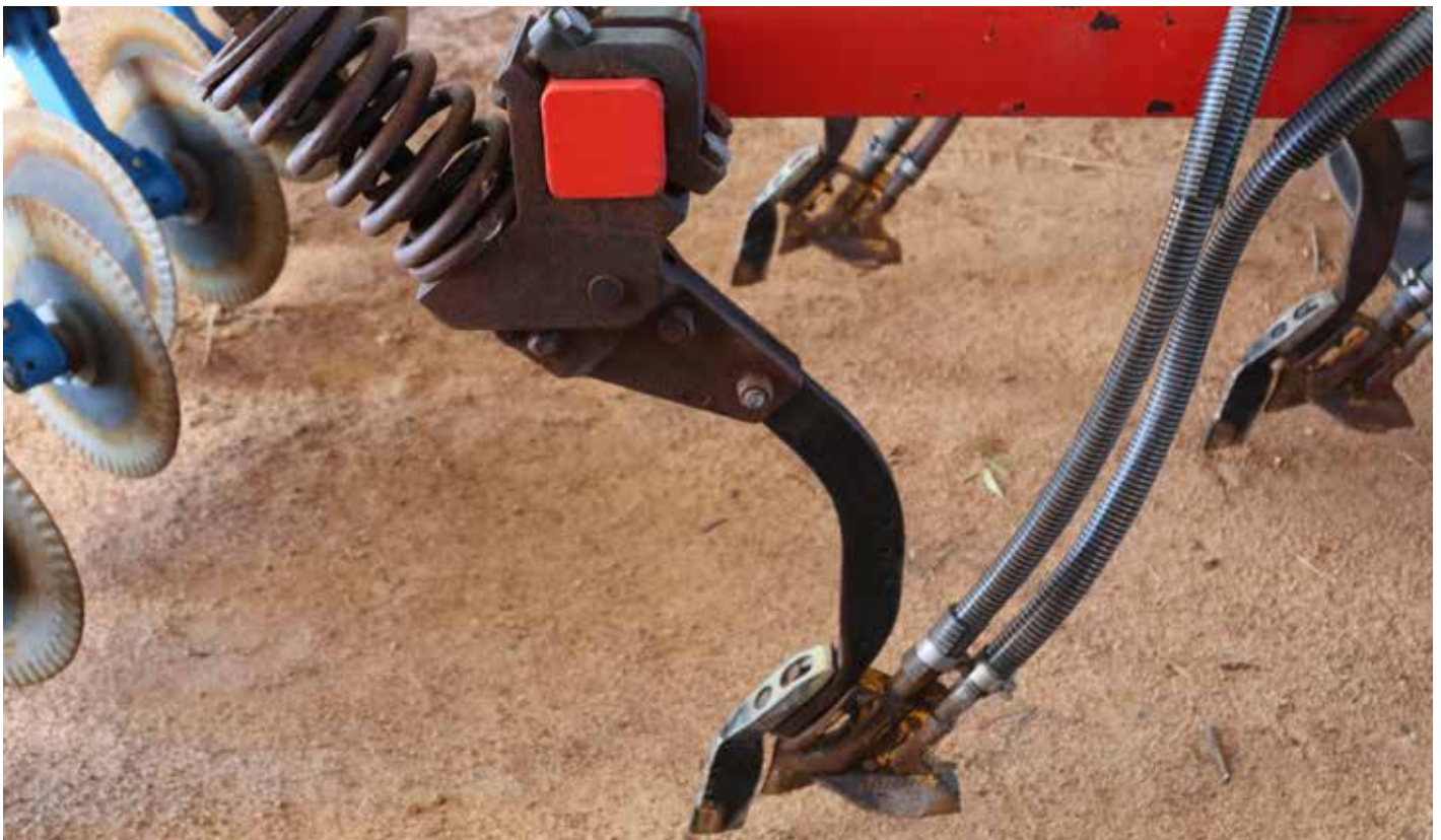
The Larkes fitted their bar with spreader plates, which allow them great flexibility in their fertiliser placement. In wet years they may choose to spread 25 per cent of the urea out the front or they could block off all the other ports and put all the urea out the front.
