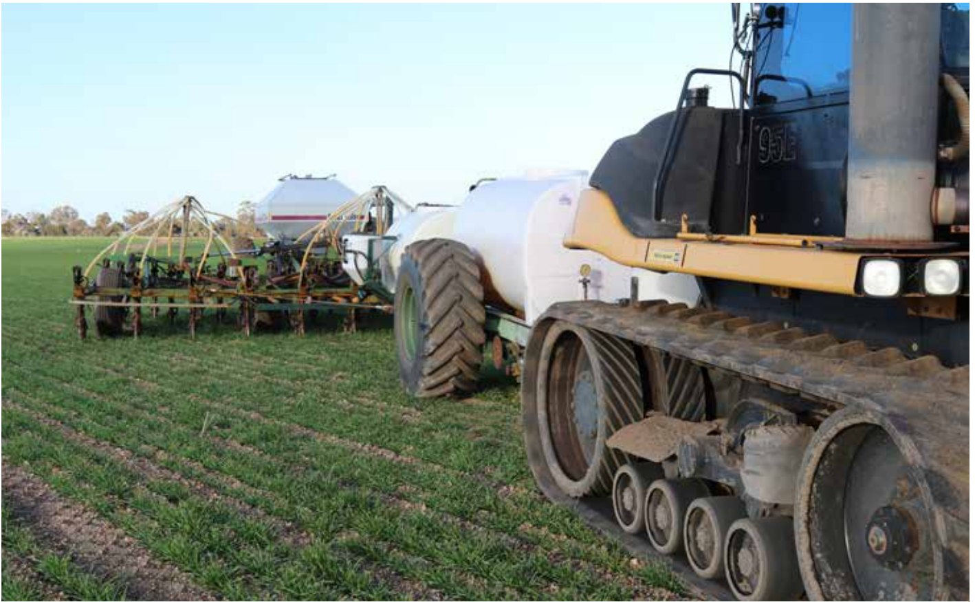
In addition to applying herbicides through the bar, the Cliftons also have a 2000L liquid injection tank to apply wetters, trace elements, liquid nitrogen and fungicides.
