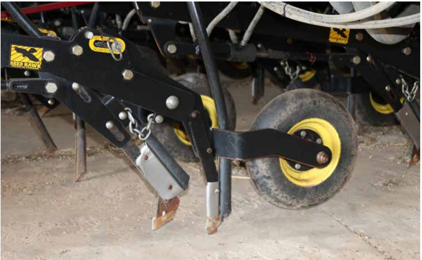
The Seed Hawk has a two-tyne set-up, with the front tyne doing most of the ripping and also deep banding urea, while the back tyne is offset 1.5-inches to the left-hand side, which puts the seed and MAP together, resulting in excellent separation of urea from the seed.
