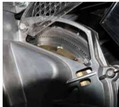
Canola seed is sucked into the small holes of the Monosem Seed Meters by a vacuum and as the plate rotates around the meter, when it gets to the drop point above the seed tube the vacuum ceases and the seed releases from the plate and drops directly through the seed tube into the ground. PHOTO: CUSSONSMEDIA
