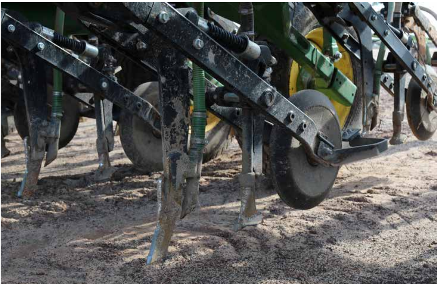
Glenn says one of the most important aspects to setting Conserva Pak up is to keep the bar level. He says, particularly in dry years, they have had problems with the machine riding forward, even with jockey wheels at the front.
