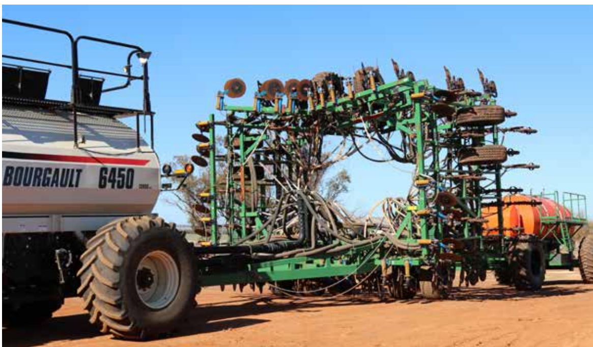
Coulters at the front of the DBS help to manage moisture and avoid blockages, particularly on dewy nights.
