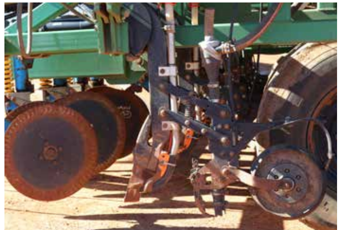
Coulters at the front of the DBS help to manage moisture and avoid blockages, particularly on dewy nights.
