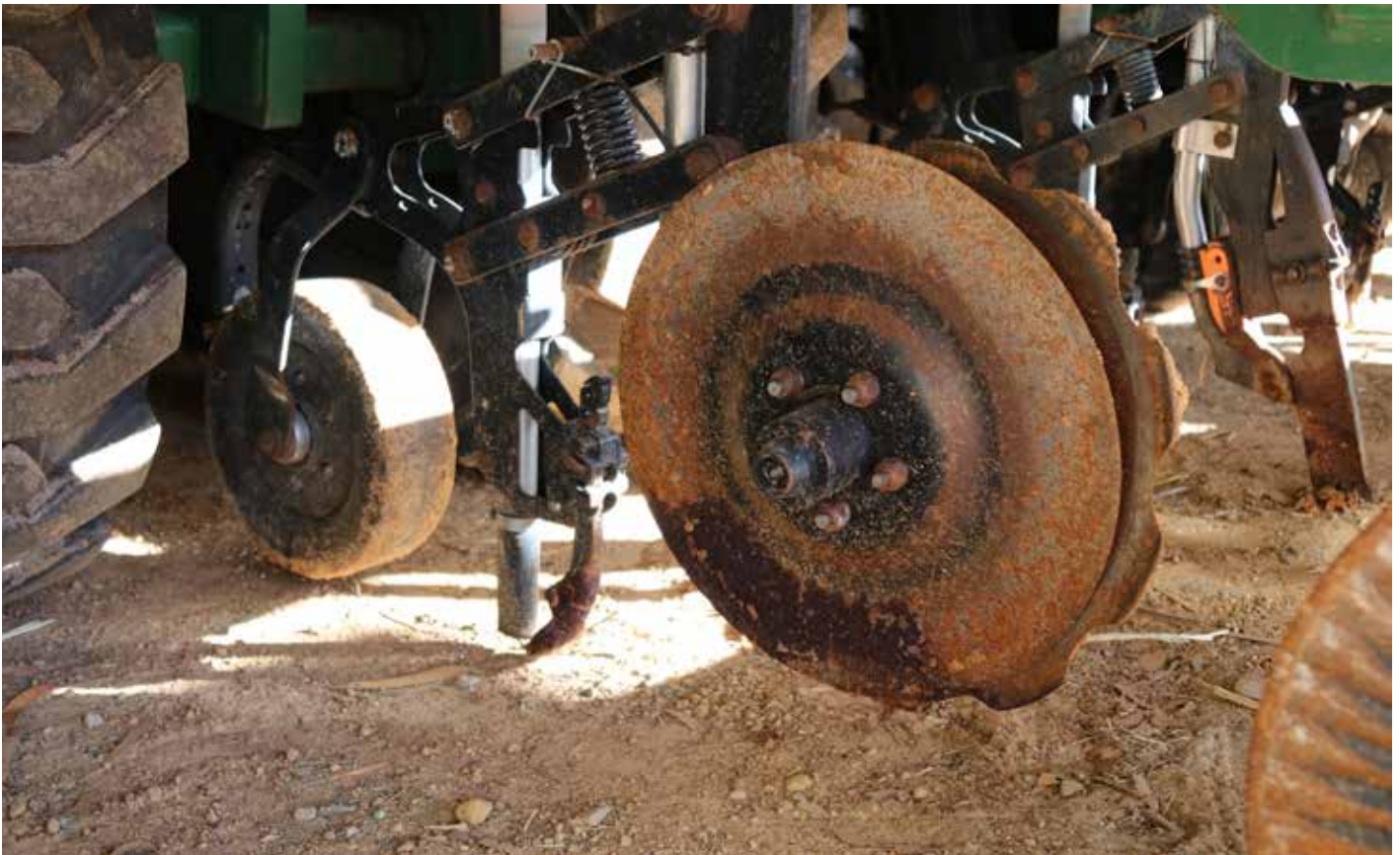
Ash has added a bolt-on disc module to prevent running tynes through his wheel tracks where he is planning to chaff deck in the 2018/19 harvest.
