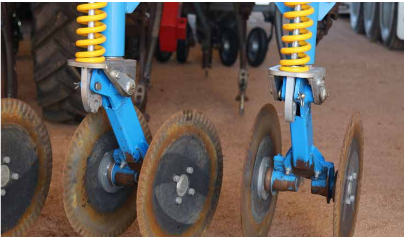
Primary Sales tandem disc coulters have been added to the front of the Scaribar to aid trash flow. The Larkes also run a Speed Tiller, which they commonly use on paddocks that are barley-on-barley to bury some of the stubble and aid its breakdown.
