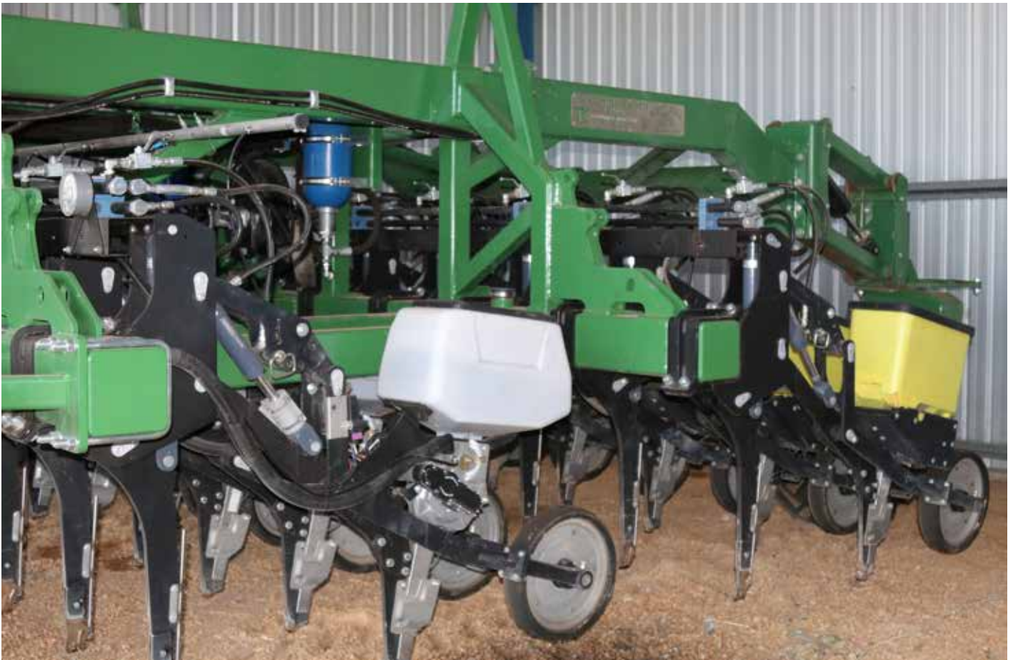
While the original version had a Precision Planter metering system (plastic plate), version two (pictured) is trialling two different seed meters and technology options. The front 10 seeder units are Monosem Seed Meters (metal plates) with Ag Leader SureDrive Electric Drives and the back 10 seeder units are Precision Planting vSet Seed Meters with Precision Planting vDrive Electric Drives.
