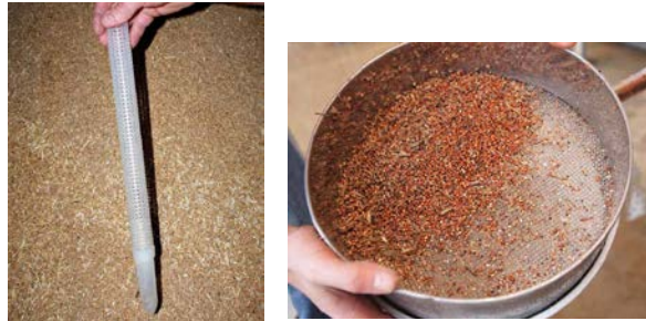
Figure 5. A probe trap (L) and an insect sieve (R) used for regular grain inspections
