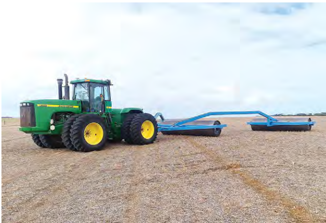
Figure 5.5: Triple-section flat steel roller, weighing up to 11 tonnes per section when filled with water.
