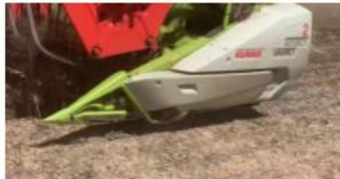
Claas Divider - multipurpose divider able to work in low and high yield crop.
