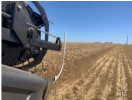
Case IH Divider - same as Macdon. Designed for high tonne crops.
