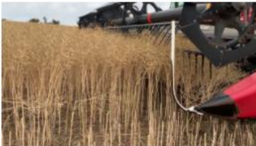
Case IH Divider - same as Macdon. Designed for high tonne crops.
