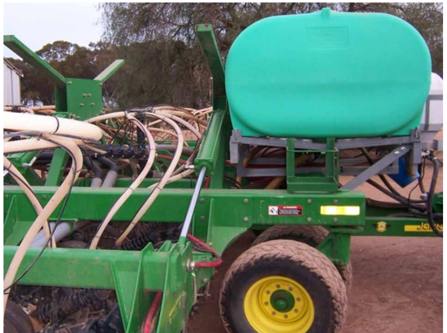
Figure 9: Tanks mounted on the seeding bar for liquid injection of rhizobia or trace elements during seeding. Agitation is required. Note the tubes and manifold. Inoculum must be applied under low pressure only. Some machines have their tanks set up as a separate, trailed tanker.
