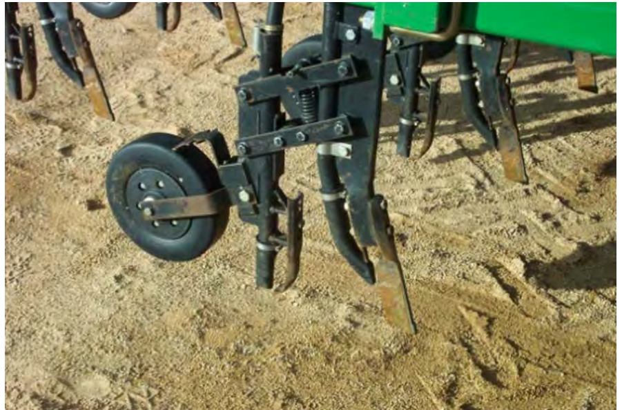
Figure 35: The DBS system parallelogram for uniform seeding depth and deep placement of seed or fertiliser.
