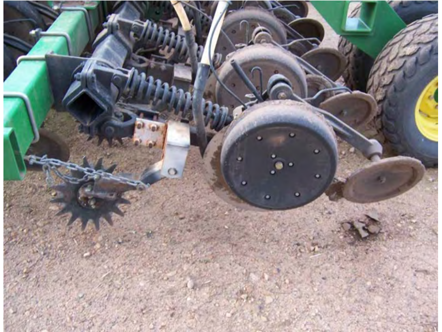
Figure 10: A disc seeder set up with Yetter trash clearing wheels and tubing for liquid injection of inoculum or trace elements during sowing. Note also the closer, to cover the seeding slot and act like a press-wheel from the side.
