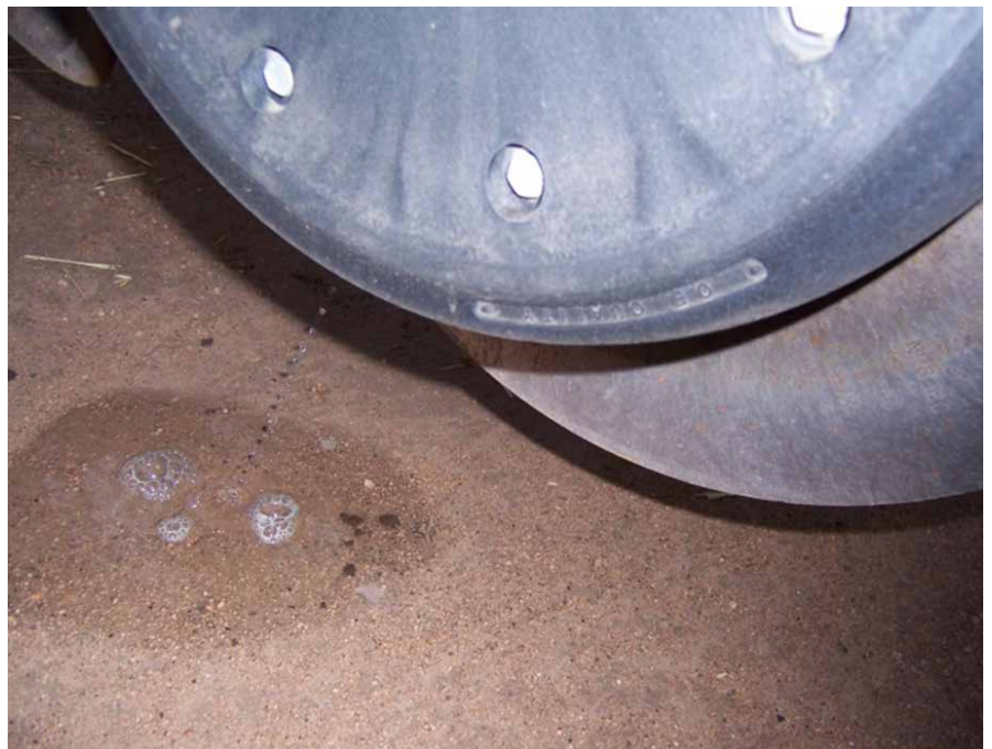
Figure 11: In-furrow liquid injection: Note the droplets from liquid injection, which can be used for inoculating pulses or applying liquid trace elements.
