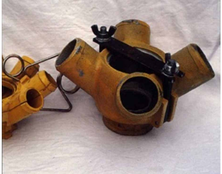
Figure 31: Conversion heads, such as this one for a Connor–Shea air seeder, allow large seeds such as faba beans and Kabuli chickpeas to be sown with ease.
