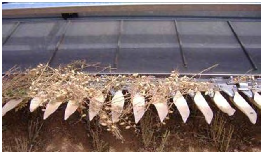
Figure 4: Plastic extension fingers fitted to a draper front.
