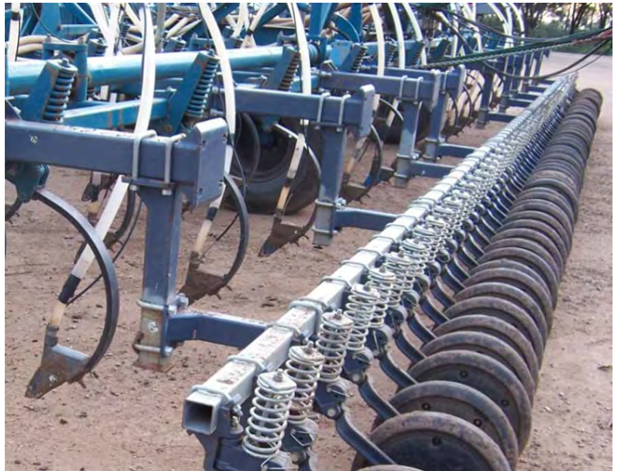
Figure 8: A seeding bar setup with Atom Jet narrow points, gang press wheels and liquid injection for either inoculum or trace element application during sowing.
