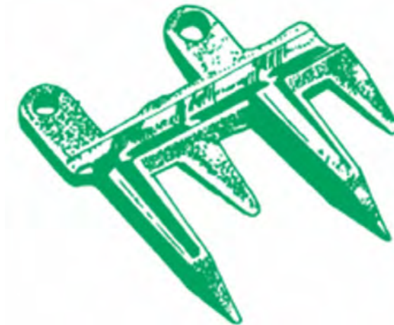
Figure 1: Four-finger guards to reduce vibration.
