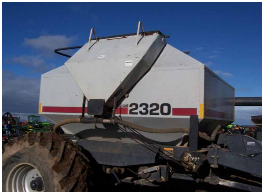
Figure 12: An ‘after-market’ third box fitted to a Flexicoil box to enable application of granular inoculum. Note that granular inoculum cannot be applied mixed with the seed (uneven distribution of seed and/or inoculums occurs). Rhizobia survival is severely jeopardised if granular inoculum is applied mixed with fertiliser.
