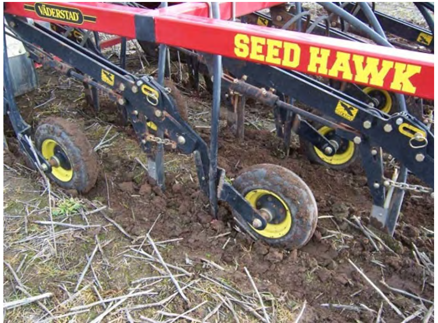
Figure 32: One of several seeding mechanisms for uniform sowing depth using the press-wheel for depth control.
