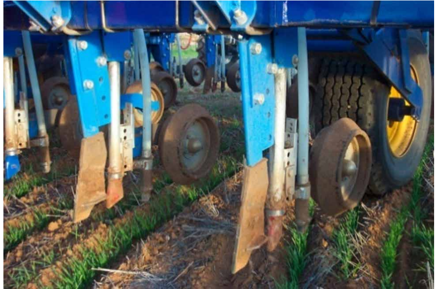
Figure 34: A primary precision seeder fitted with hydraulic breakout for consistent penetration. Also fitted are narrow points that form an 'inverted-T' slot and are capable of deep or side placement of fertiliser.
