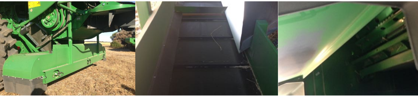
IMAGES (L-R) (1) Mick's chaff deck. (2) The belt running across the back of the machine, showing the cover between the left and right side belt. (3) The baffle/dividing plate to separate the chaff from the straw. Note the 'bull nose', designed to minimise stems lodging on the leading edge.
