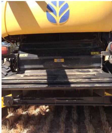
IMAGES: The conveyor belt is continuous, and runs at 90° to the direction of travel.
