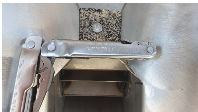
Figure 1. Metering unit for amendment application on the Qld research machine, with ruler for scale.
