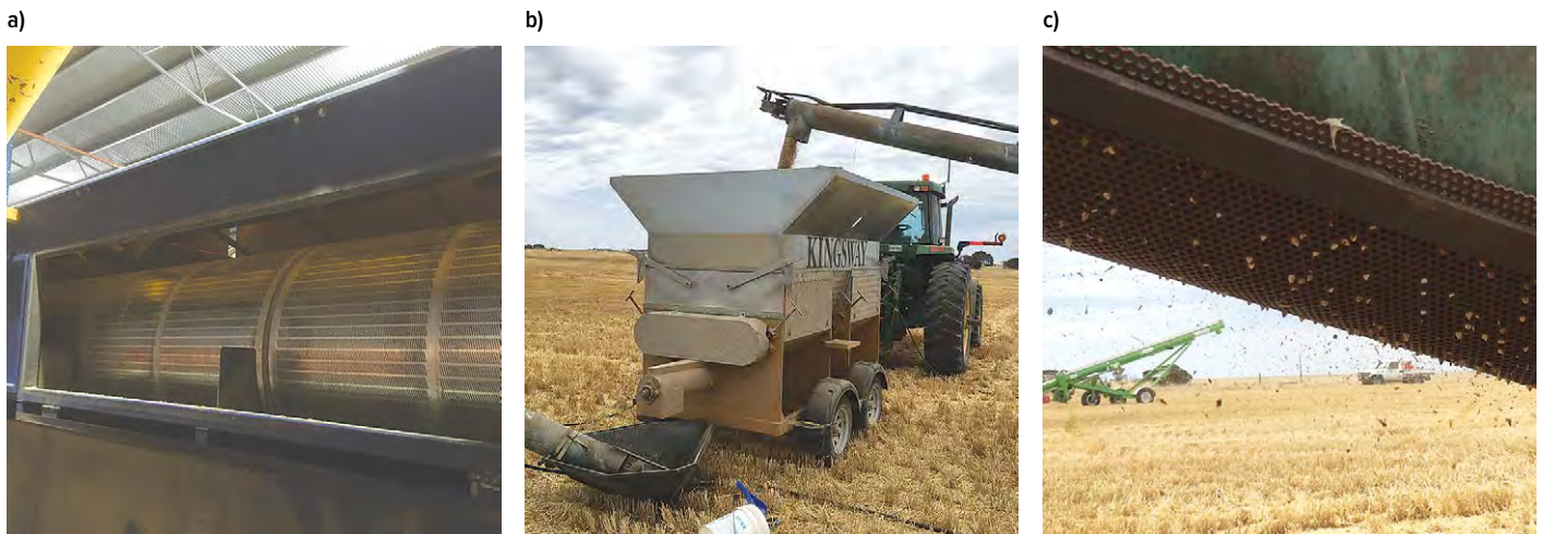
Figure 6.2: a) Rotary cleaner, b) snail-crushing roller and c) auger fitted with lower screens to remove small snails and fragments.
