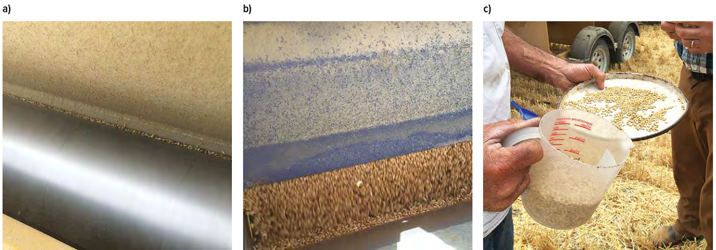
Figure 6.3: a) and b) Snail rollers and c) monitoring the rolling operation.
