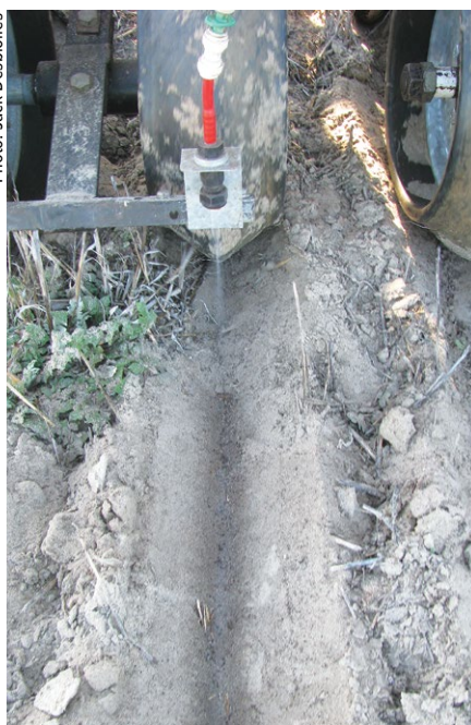
Figure 2: Application of soil wetter behind water-harvesting ‘open V’ press-wheels via a narrow (15 degree) flat fan nozzle achieving a stable 3cm wide spray footprint at the base of a firm furrow.
