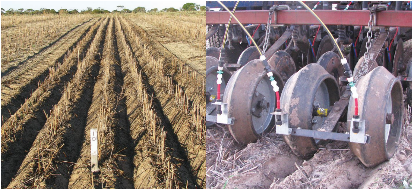
Figure 1: Water-harvesting stable furrows (left) shaped by wide V-shouldered press-wheel tyres (right) help soil wetter effectiveness, while maintaining standing stubble is often best practice for minimising furrow infill over time.
