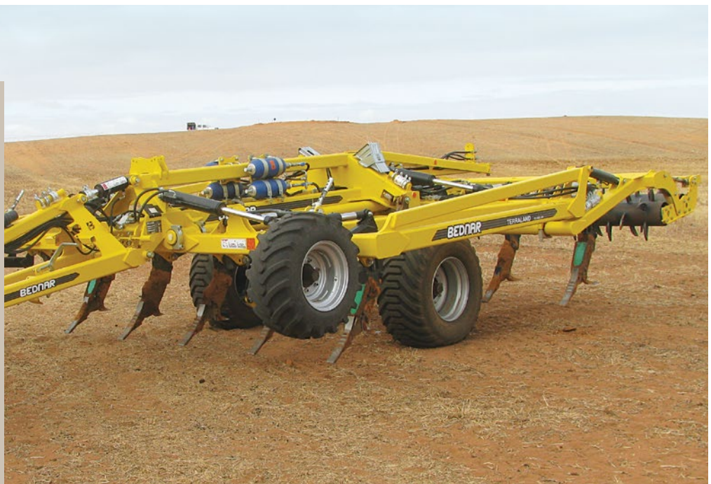
Photo 1: High disturbance ripper using narrow-spaced delving tynes to bring up soil from deeper layers combined with levelling spike rollers to provide a levelled finish.
