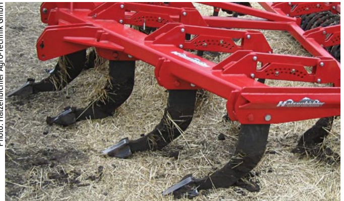
Photo 2: Parabolic narrow shank ripper fitted with winged high lift points for maximum soil loosening depth capacity.
