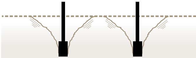
Figure 3: Impact of tyne spacing on soil disturbance pattern. Note: the undisturbed dome or ridge between rip lines represents a loosening gap relative to the targeted area of spacing x depth while the optimum tyne spacing is also affected by ripping depth.
