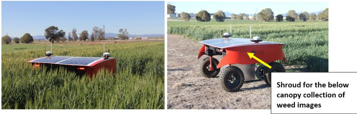
Figure 2. Autonomous platform with suspended shroud containing a digital image collection system and a constant light source.
