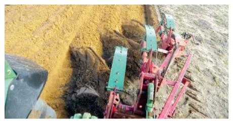
**Photo 7:** The impact of tilling varies with the implement used: inversion tillage using a mouldboard plough, as pictured here, results in greater impacts than using a chisel or disc plough.
