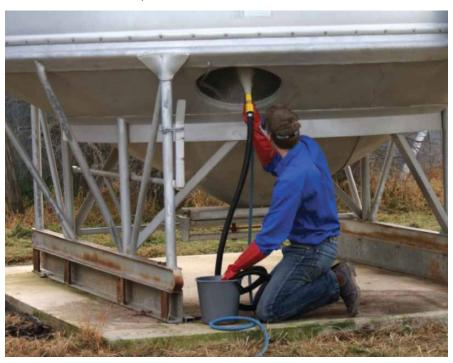
**Photo 9:** A blower and vacuum gun such as the Venturi gun is the best applicator for inert dusts. Aim for an event coat of diatomaceous earth across the roof, walls and base.
