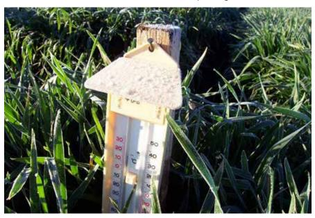
**Photo 7:** Canopy temperature measured using a calibrated minimum—maximum thermometer. For best results, a minimum of two or three field thermometers are required to give representative temperatures for a crop. In undulating country, more thermometers should be used to record temperatures at various heights in the landscape.
