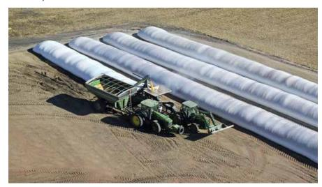
**Photo 3:** A 100 m bag can be filled in 30 minutes when there is a constant supply of grain.
